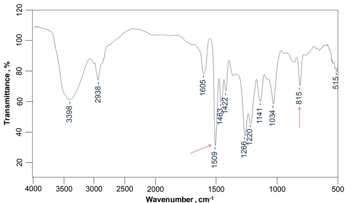
**Figure 4.** IR spectrum of the softwood derived lignophenol. The arrows emphasize the distinctive bands related to its chemical structure
