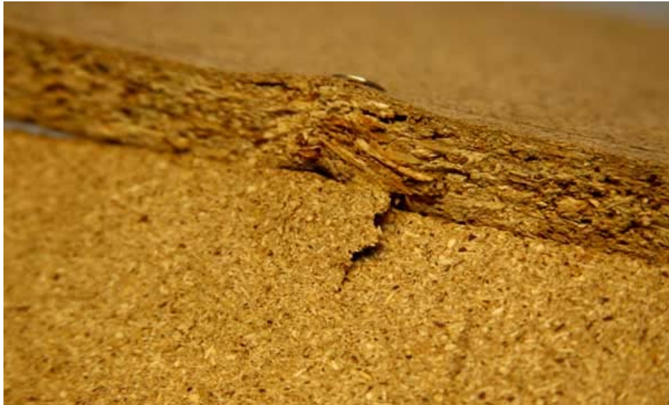
Fig. 14. The damage form of the connection with confirmat
