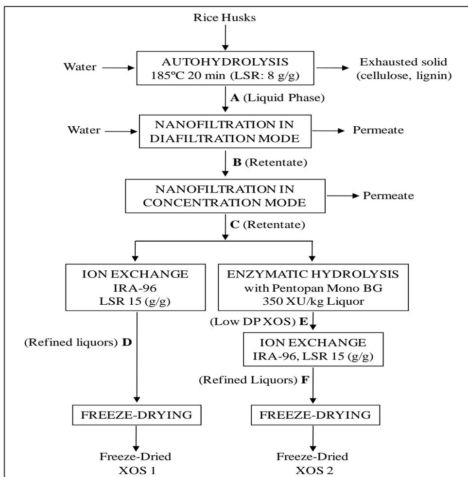
**Fig. 1.** Scheme of the process employed in this work for obtaining purified xylooligosaccharide concentrates
