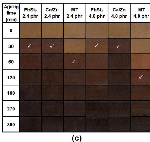
**Figure 5.** Digital photographs for neat PVC and WPVC composites containing PbSt<sub>2</sub>, Ca/Zn and MT at dosage of 2.4 and 4.8 phr: wood flour at (a) 0 phr, (b) 50 phr and (c) 70 phr
