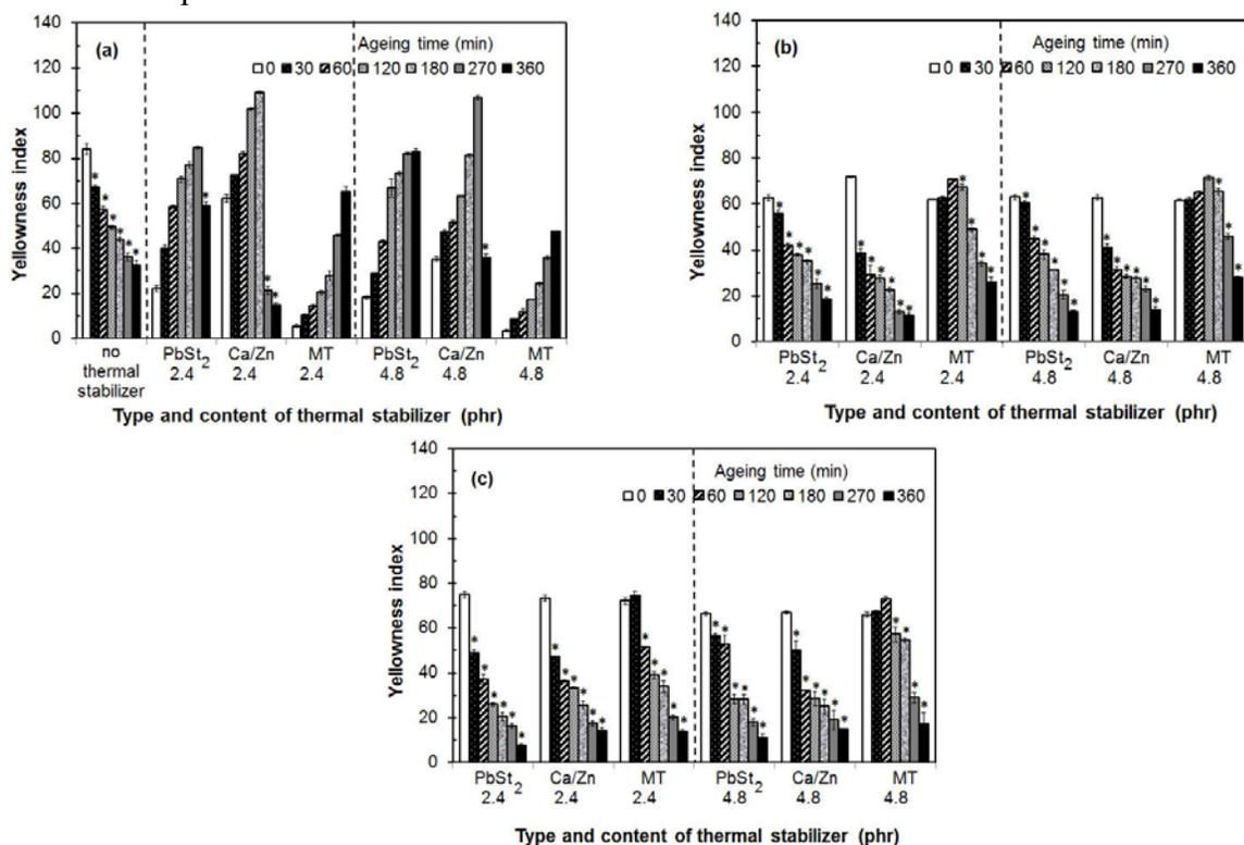
**Figure 4.** Yellowness index of neat PVC and WPVC composites with three thermal stabilizers at different ageing times at 177°C : wood flour at (a) 0 phr, (b) 50 phr, and (c) 70 phr (\* specimens turning dark color)
