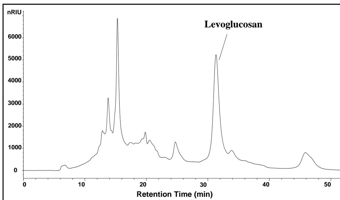
**Fig. 2.** Liquid chromatogram of a typical bio-oil aqueous fraction sample
