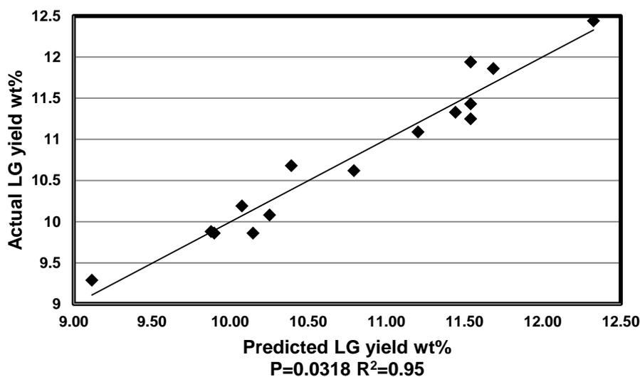
**Fig. 4.** The relationship between the actual and predicted levoglucosan yield extracted into the aqueous fraction as predicted by regression analysis
