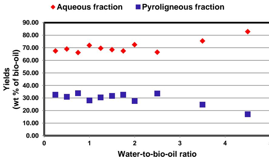
Fig. 1. Effect of the water-to-bio-oil ratio on the yields of aqueous and pyrolygneous fractions
