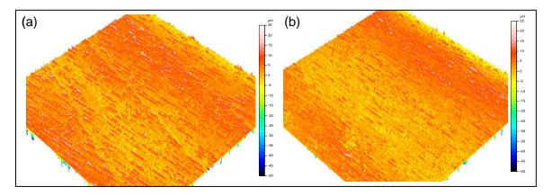
**Fig. 8.** 3D Renderings of profilometric measurements on edge-glued yellow birch panels (a) with a water-based stain (b) with a solvent-based stain. Color scale goes from -50  $\mu$ m to 25  $\mu$ m Surface dimensions: 20 x 20 mm
