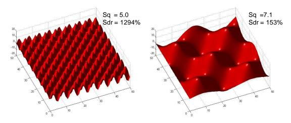
Fig. 1. Comparison of roughness parameters for two hypothetical surfaces
