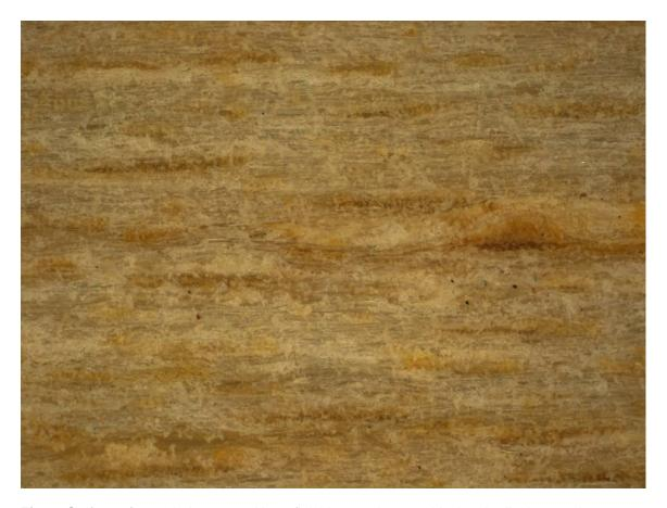
Fig. 4. Surface of a peeled veneer without finishing products and its longitudinal parenchyma
