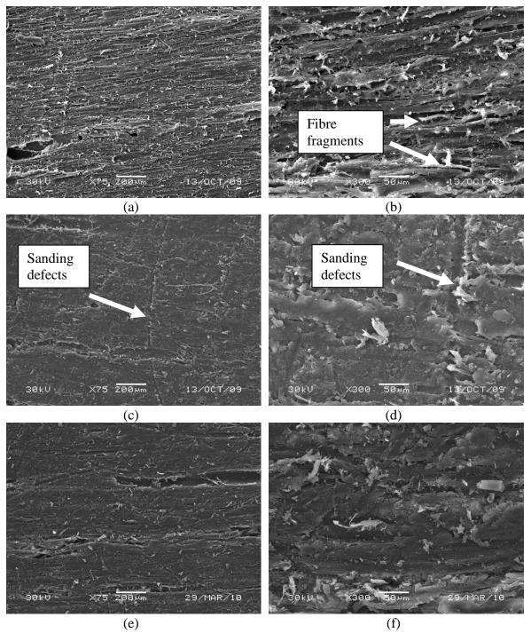
**Fig. 6.** Veneer samples stained with a water-based stain (a, b); solvent-based stain (c, d) and untreated samples (e, f)
