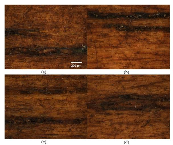
Fig. 3. Images of stained surfaces (a) lumber with a water-based stain; (b) lumber with a solvent-based stain; (c) veneer with a water-based stain; (d) veneer with a water-based stain
