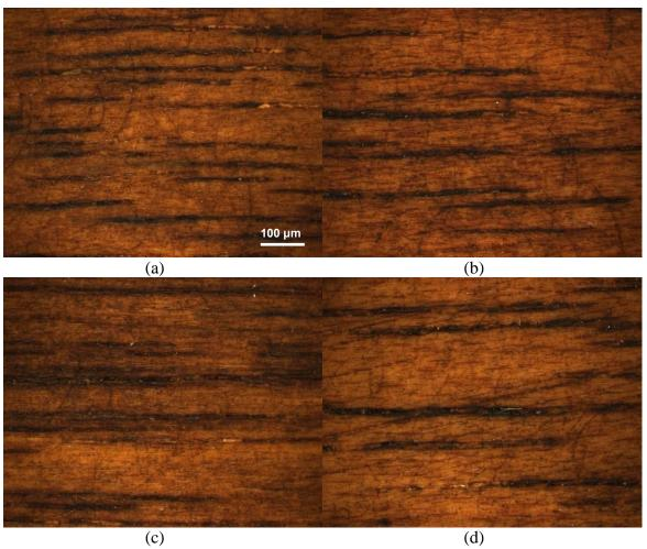
Fig. 2. Images of stained surfaces (a) lumber with a water-based stain; (b) lumber with a solvent-based stain; (c) veneer with a water-based stain; (d) veneer with a water-based stain
