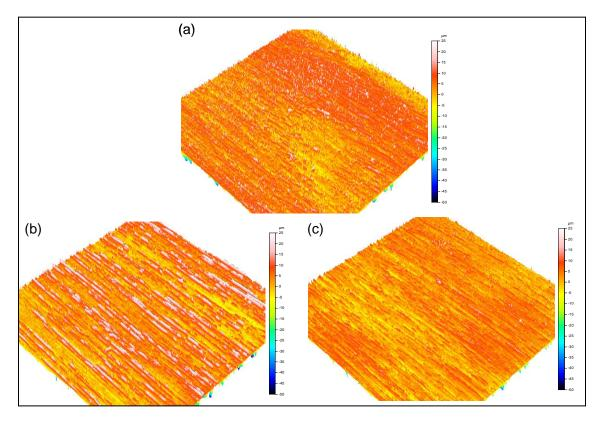
**Fig. 7.** 3D Renderings of profilometric measurements on sanded veneer without finishing products (a); with a water-based stain (b); with a solvent-based stain (c). Color scale goes from -  $50 \mu m$  to  $25 \mu m$  Surface dimensions:  $20 \times 20 mm$
