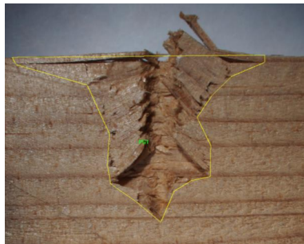
Fig. 2. Measuring method for the fractured area using a polygon-shaped area
