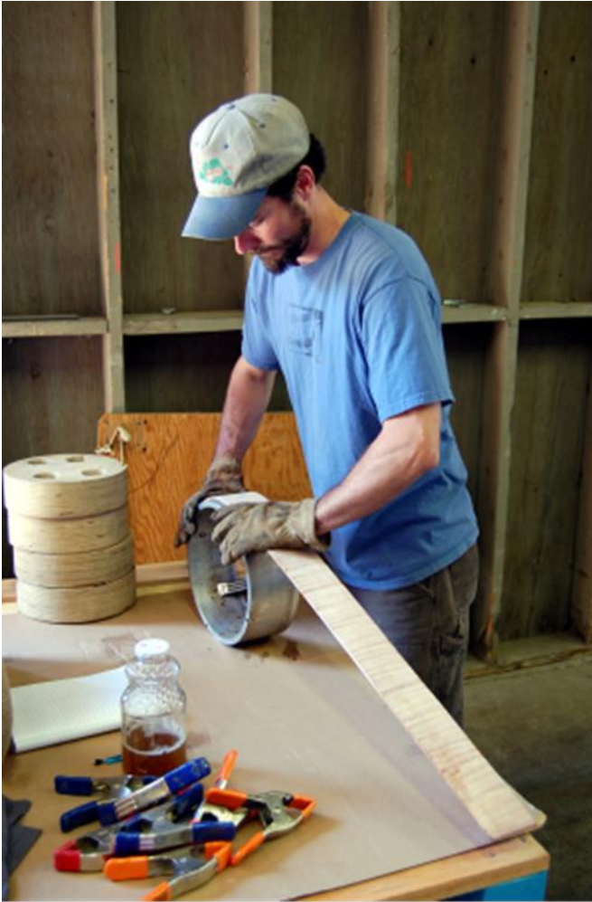
Fig. 2. Greg Galbreath, luthier and "Buckeye Banjos" owner bends steamed curly maple around hoop mold. Cooling forms stacked on left, which formed hoops are clamped to. The drink is ice tea! Photo by author 2008
