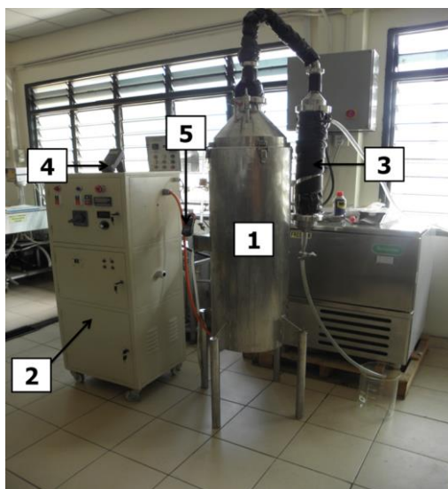
Fig. 1. The ohmic-heated hydro-distillation system: (1) ohmic-heated hydro distiller unit, (2) power supply, (3) multi-tube condenser unit, (4) temperature sensor, (5) clamp meter
