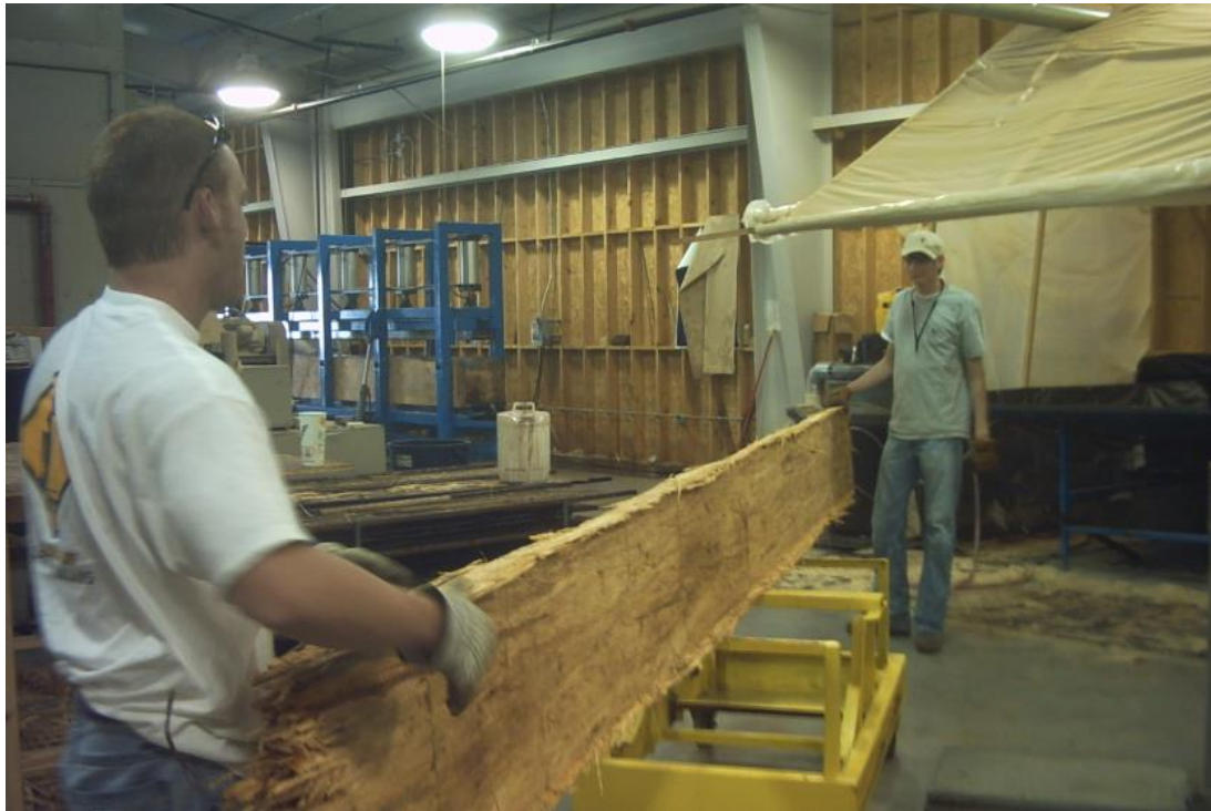
Fig. 1. Typical rough beam shown immediately after pressing
