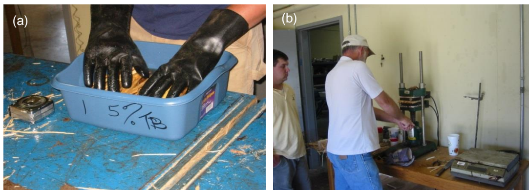
Fig. 3. (a) Treating scrim in GP resin blended with 5% DOT, (b) pressing a 6 in × 6 in mat
