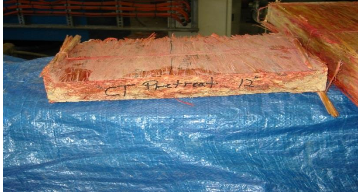
Fig. 4. Penetration of silane-based WRP (dyed red) in a beam formed using scrim treated prior to pressing
