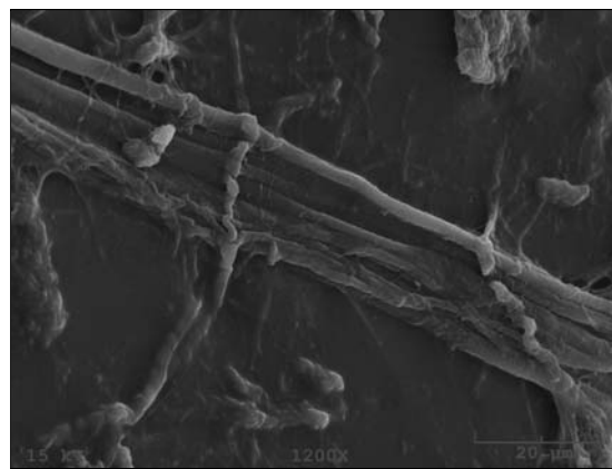
Fig. 5. OS1 fungal treatment of fibres, (a) fungus growing on the fibre, (b) treated fibre before high shear refining
