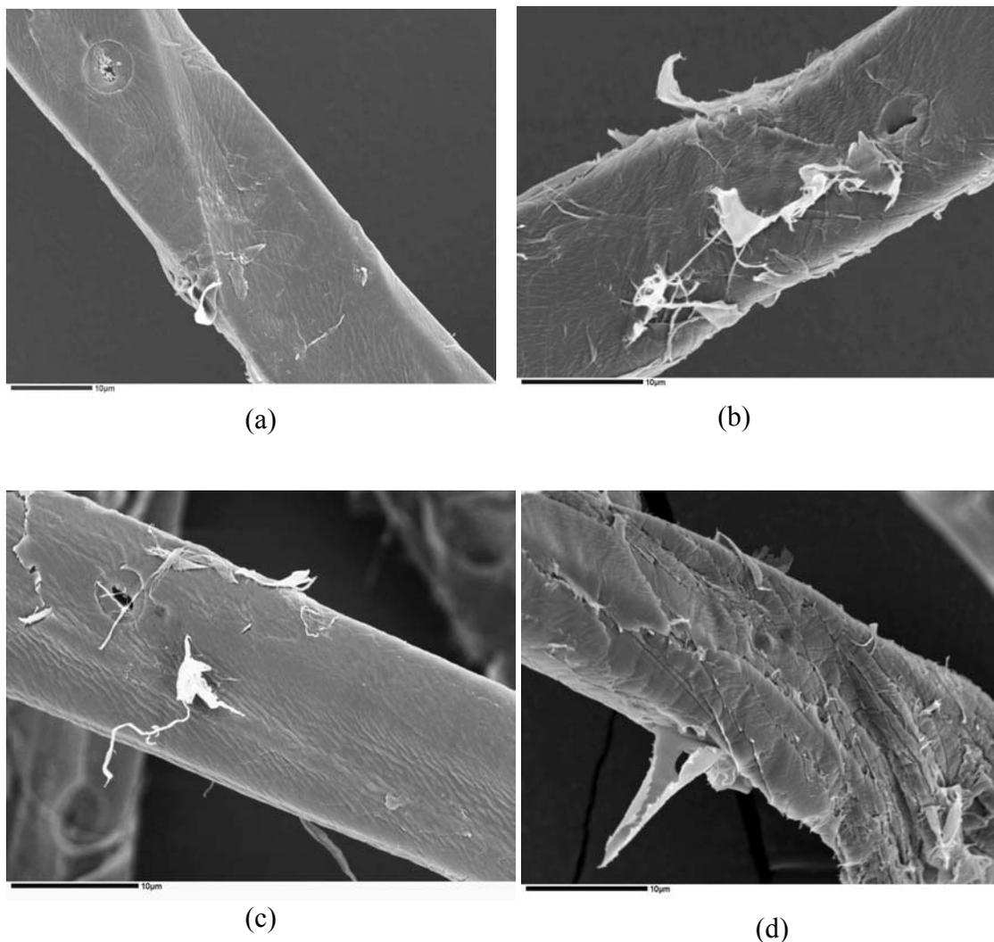
**Fig. 2.** SEM images of eucalyptus CTMP fibers before and after *T.h*-19-6 fungal treatment. (a) image of a control CTMP fiber; (b) a control CTMP fiber after PFI treatment; (c) a fungal-treated CTMP fiber; and (d) a fungal-treated CTMP fiber after PFI treatment.
