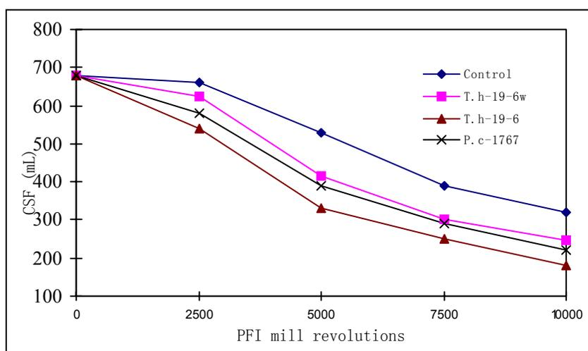
**Fig. 1.** Freeness change PFI mill revolutions of the control and fungal-treated eucalyptus CTMP pulps.
