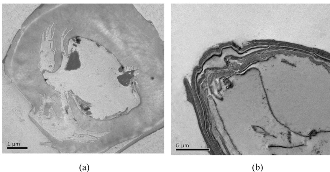
**Fig. 3.** TEM images of eucalyptus CTMP fibers after T.h-19-6 fungal treatment. (a) without PFI refiner treatment; and (b) after PFI treatment.
