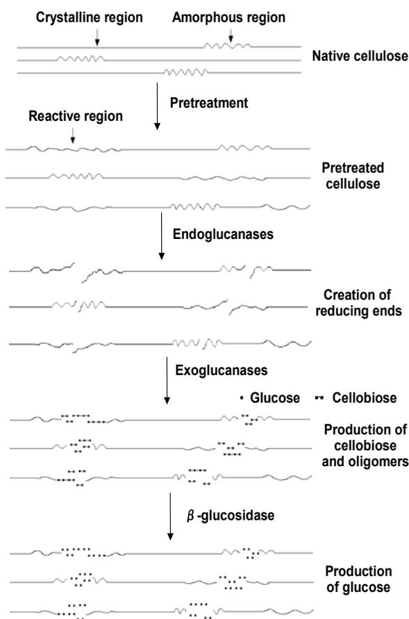
**Fig. 2.** Schematic presentation of hydrolysis of cellulose to glucose by cellulolytic enzymes.
