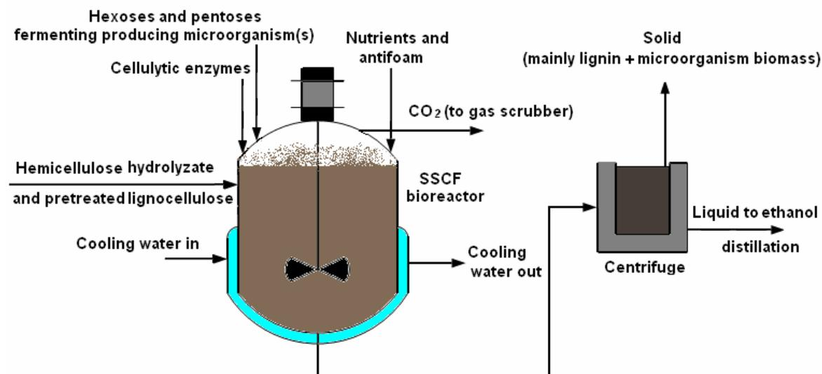
**Fig. 6.** Simplified process flow diagram for simultaneous saccharification and cofermentation (SSCF)
