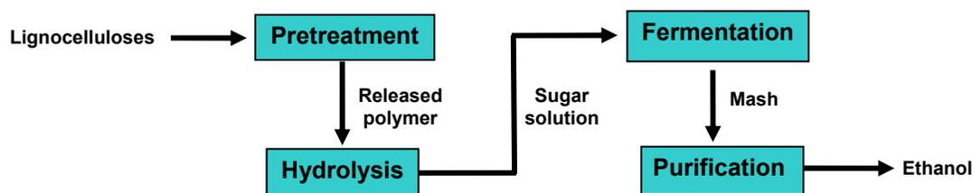
**Fig. 1.** Different units in the main line of ethanol production from lignocellulosic materials
