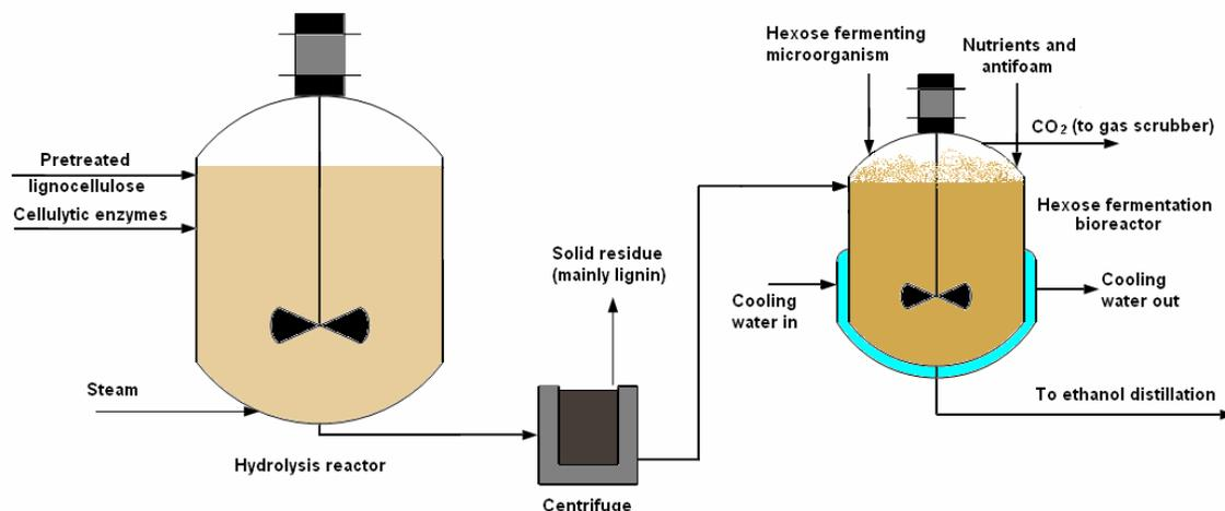
**Fig. 5.** Simplified process flow diagram for nonisothermal simultaneous saccharification and fermentation process (NSSF)
