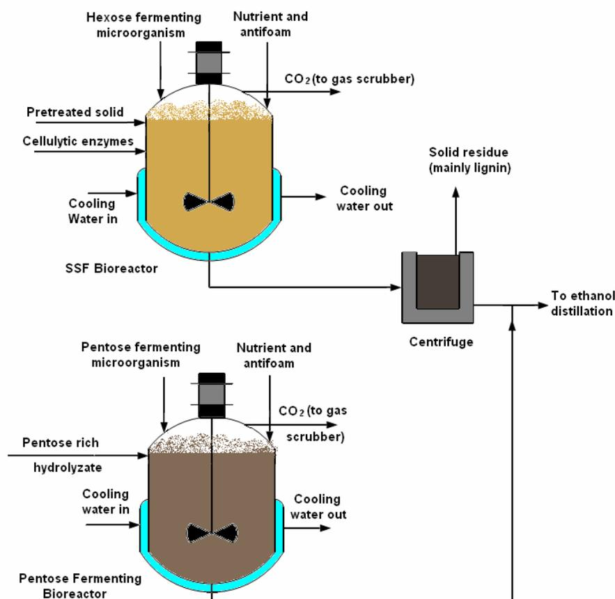
**Fig. 4.** Simplified process flow diagram for simultaneous saccharification and fermentation
