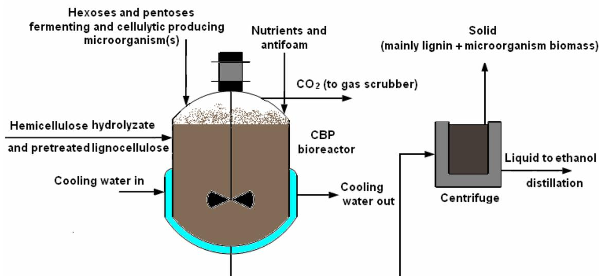
Fig. 7. Simplified process flow diagram for consolidated bioprocessing (CBP)
