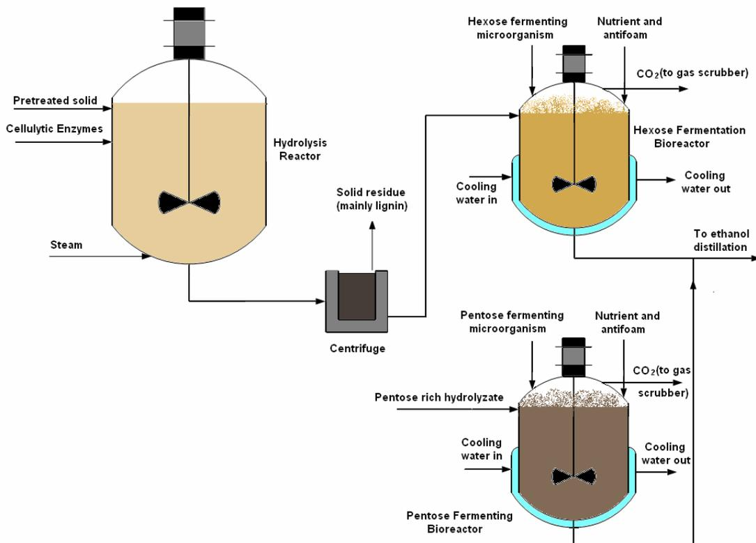
Fig. 3. Simplified process flow diagram for separate enzymatic hydrolysis and fermentation (SHF)
