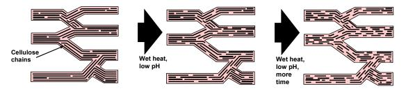
**Figure 6.** Schematic illustration of hydrolytic cleavage of cellulose chains within a "fringed micelle" structure of cellulose in a kraft fiber cell wall. A small amount of hydrolysis may go unnoticed, but eventually the fibers become brittle and susceptible to mechanical damage (Kato and Cameron 1999).
