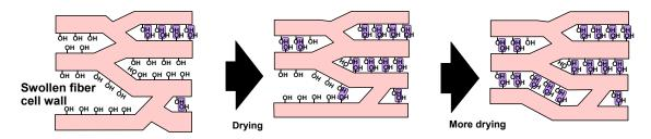
**Figure 5.** Schematic diagram of mechanism by which the "zipping" shut of pores is mediated by highly orderly hydrogen bonds, resulting in crystalline micro-domains that resist separation. Interfibril hydrogen bonds are shown with shading.
