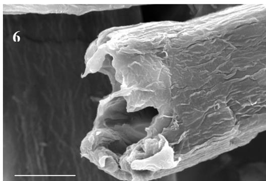
**Figs 4-6.** Three stages in HCl attack on softwood spruce fibres. **Fig. 4:** Initial degradation of the S1 wall. **Fig. 5:** Further attack cleaving both the S1 and S2 fibre walls. **Fig. 6:** Complete cleavage of the fibre, also revealing the cell lumen. Bar: 10 µm.
