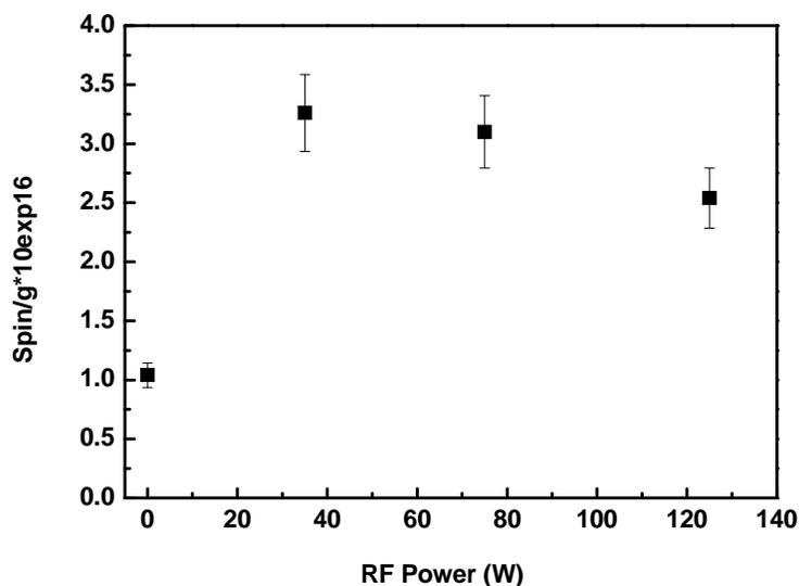
**Fig. 2.** Concentration of phenoxy radicals in CTMP fibers as a function of RF power, at 0.4 mbar Ar pressure, 4 pulses of 30 s.
