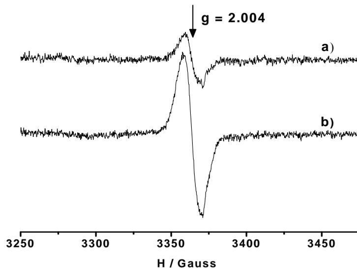
**Fig. 1.** X-band EPR spectra recorded at 123 K on CTMP fibers a) untreated and b) after plasma treatment at 0.4 mbar pressure, 75 W RF power and 2 pulses of 30 s.
