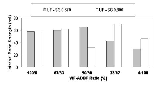
Figure 4. Effects of various WF and ADBF fiber mixtures and fiberboard density on internal bond strength (IB)
