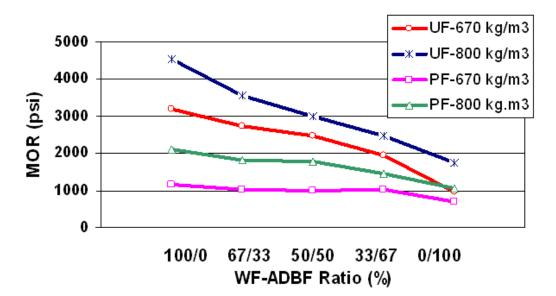
**Figure 3.** Effects of various WF and ADBF fiber mixtures and fiberboard density on Modulus of Rupture (MOR)
