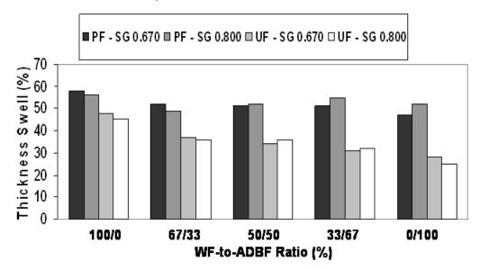
**Figure 5.** Effects of various WF and ADBF fiber mixtures and fiberboard density on thickness swell (TS) after 24-hr soak
