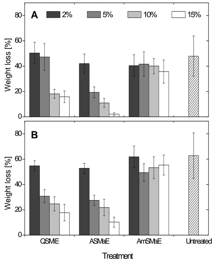
Figure 2: Mass loss of pine mini-bocks caused by *Coniophora puteana* (A) and of beech mini-bocks caused by *Trametes versicolor* (B) after 12 weeks incubation according to Bravery (1978)
