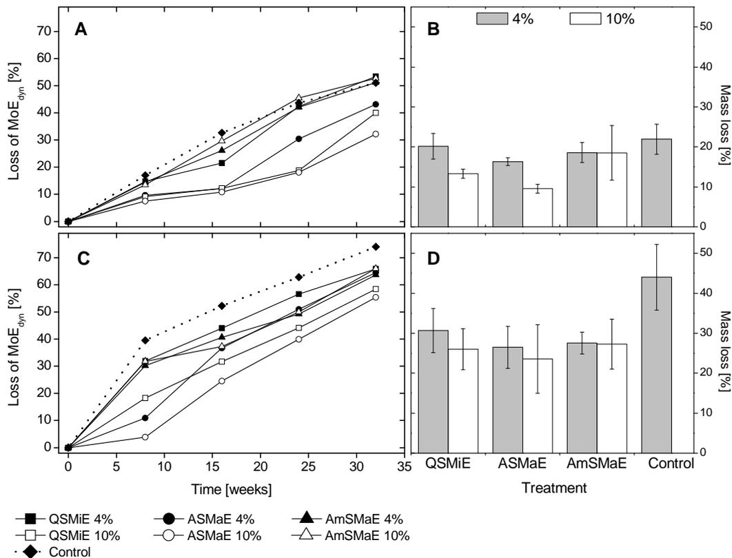
**Figure 3:** Loss of dynamic MOE of pine sapwood (A) and beech wood (C) during 32 weeks exposure in a soil bed according to ENV 807 and final weight at the end of the exposure (B: pine sapwood; D: beech)
