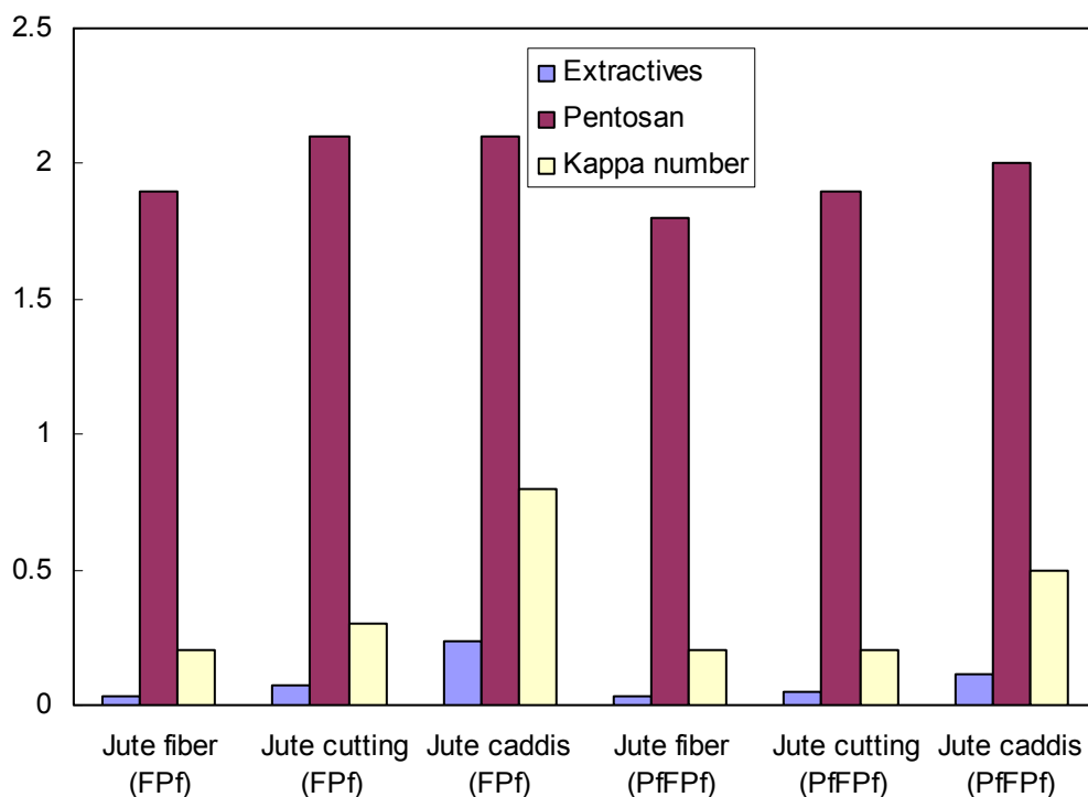
Fig. 4. Kappa number, extractives, and pentosan content of final pulps
