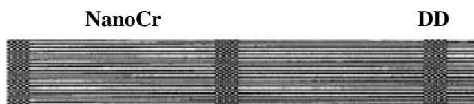
Figure 5. Elementary nanofibril of cellulose: NanoCr – nanocrystallite; DD-disordered domain
