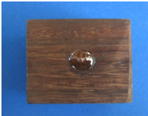
Fig. 9. Determination of heat-treated wood wettability. Original photograph
