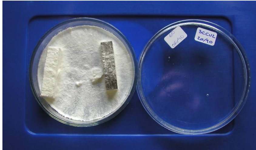
Fig. 5. Heat-treated wood (right sample) resistance to fungal attack in relation to untreated wood (Left sample). Adapted from Esteves (2006)
