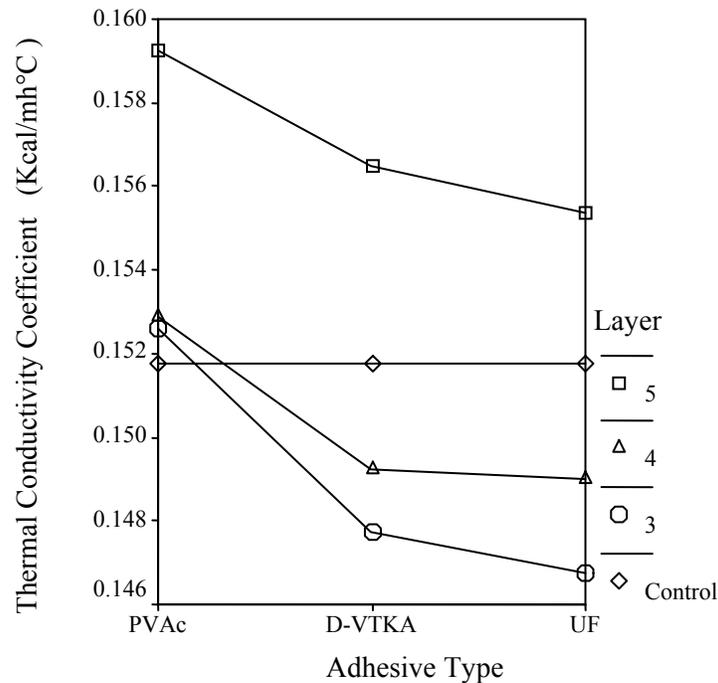
**Figure 4.** Effect of types of adhesives and layer in LVL on TC in oriental beech
