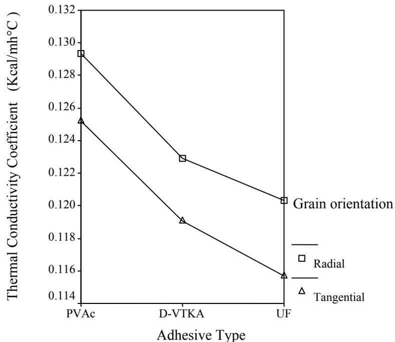
**Figure 1.** Effect of types of adhesives and grain orientation on thermal conductivity in Scotch pine
