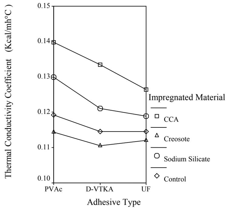
Figure 5. Effect of types of adhesives and impregnated material on TC in Scotch pine
