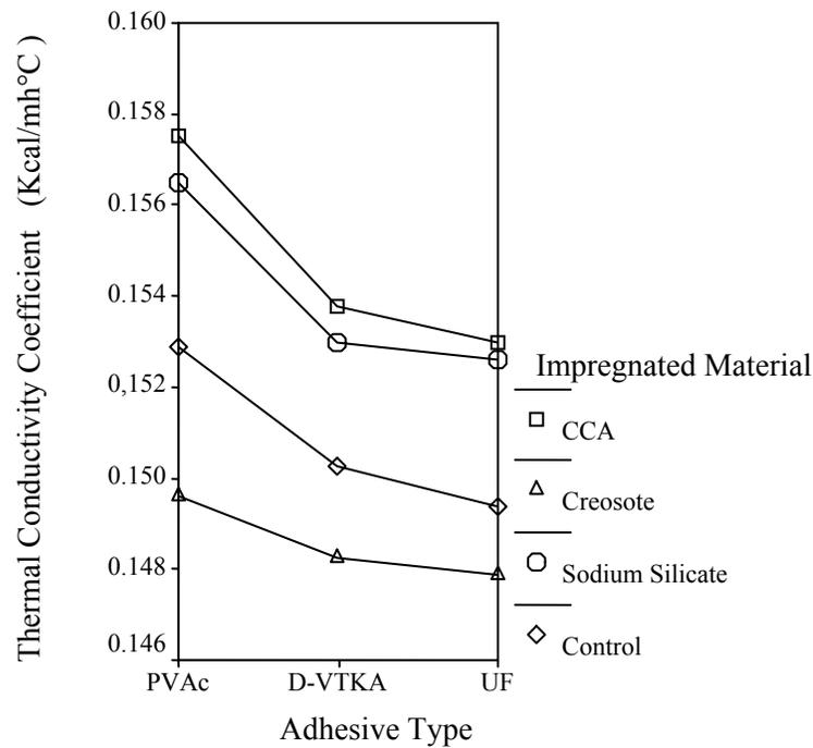
Figure 6. Effect of types of adhesives and impregnated material on TC in O. beech
