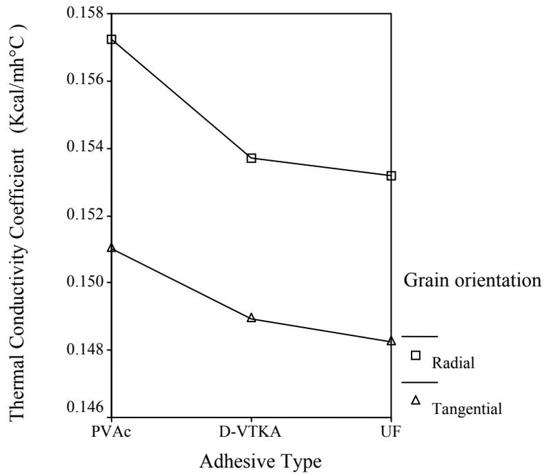
**Figure 2.** Effect of types of adhesives and grain orientation on  $T_c$  in oriental beech; thermal conductivity in radial direction are at average 5- 10 % higher than the ones in tangential direction (Ors and Keskin 2001).
