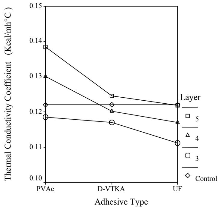
**Figure 3.** Effect of types of adhesives and layer in LVL on TC in Scotch pine
