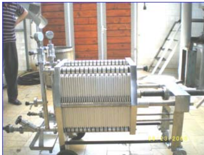
Fig. 3. Equipment used in industrial filtration of wine
