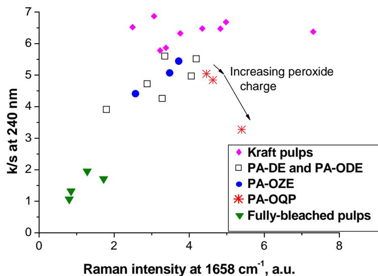
**Fig. 15.** Correlation of UV-Vis absorption band at 240 nm to Raman band at 1658 cm<sup>-1</sup>.
