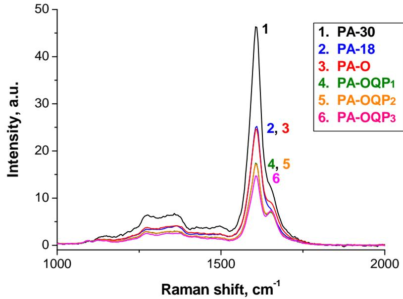
**Fig. 8.** UVR spectra of profiled alkaline-cooked (PA) pulps bleached with hydrogen peroxide. Peroxide charge increased in order PA-OQP<sub>1</sub><PA-OQP<sub>2</sub><PA-OQP<sub>3</sub>.
