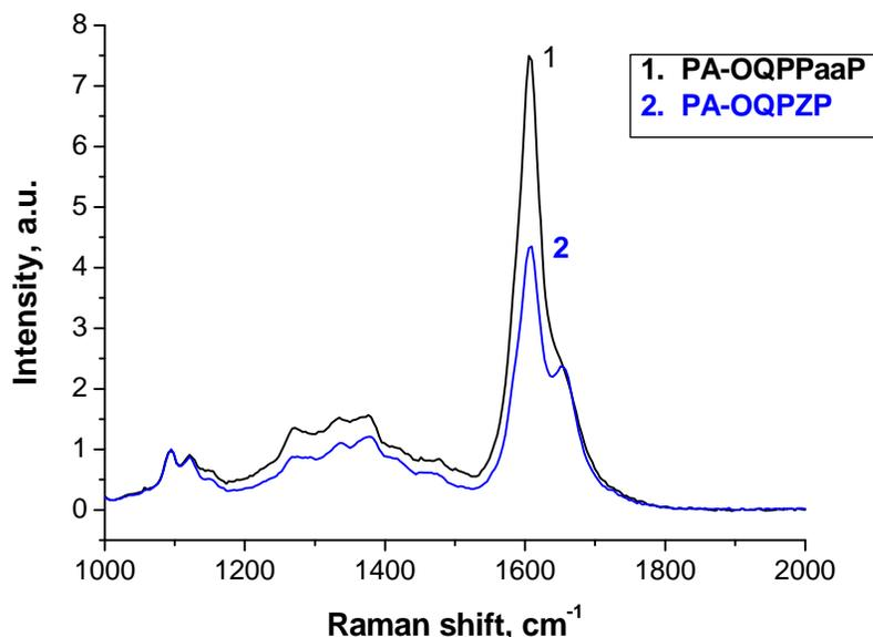
**Fig. 10.** UVRR spectra of PA-OQPPaaP and PA-OQPZP pulps.
