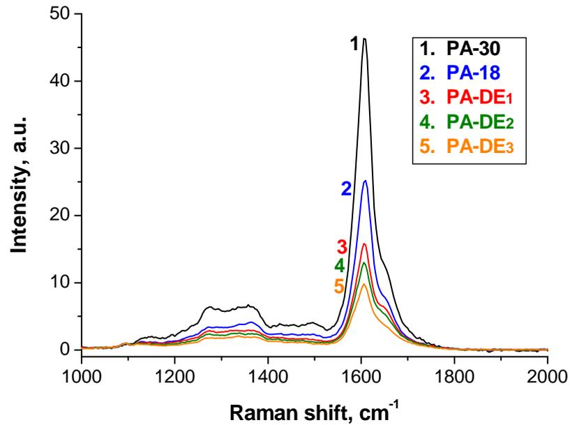
**Fig. 6.** URRR spectra of profiled alkaline-cooked (PA) pulps at two different kappa levels (kappa 30 and 18) before and after chlorine dioxide bleaching. Chlorine dioxide charge increased in order  $PA-DE_1 < PA-DE_2 < PA-DE_3$ .
