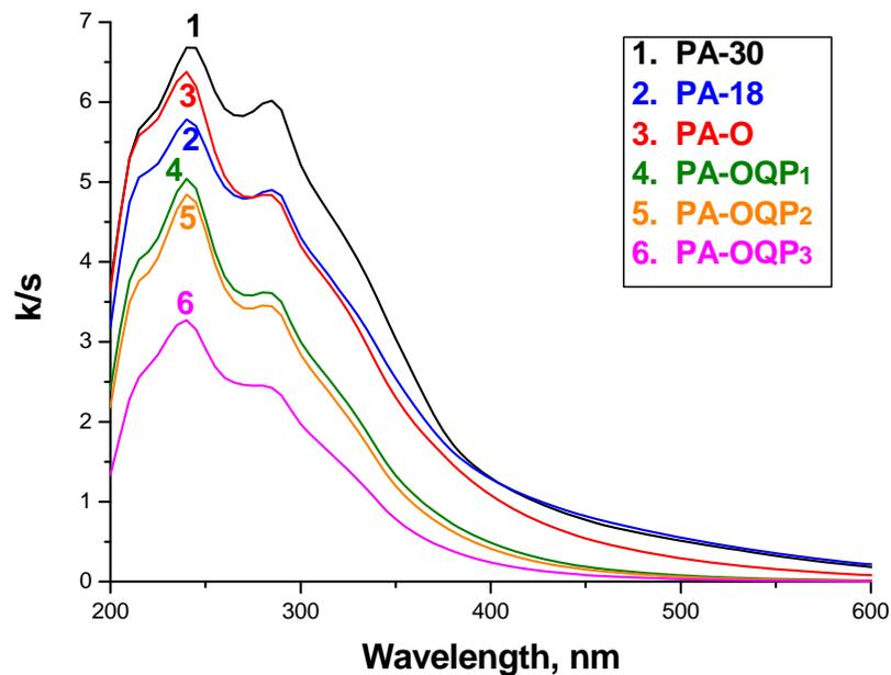
**Fig. 9.** UV-Vis spectra of profiled alkaline-cooked (PA) pulps bleached with hydrogen peroxide, converted into  $k/s$  curves. Peroxide charge increased in order PA-OQP<sub>1</sub><PA-OQP<sub>2</sub><PA-OQP<sub>3</sub>.
