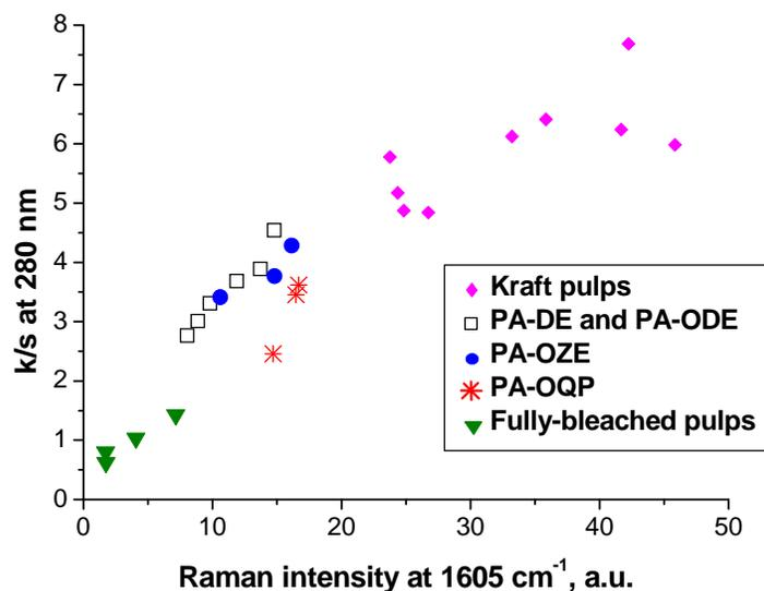
**Fig. 14.** Correlation of UV-Vis absorption band at 280 nm to Raman band at 1605 cm<sup>-1</sup>.
