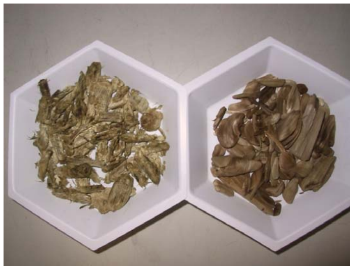
Fig. 15. The physical appearance of knot rejects before and after enzymatic hydrolysis
