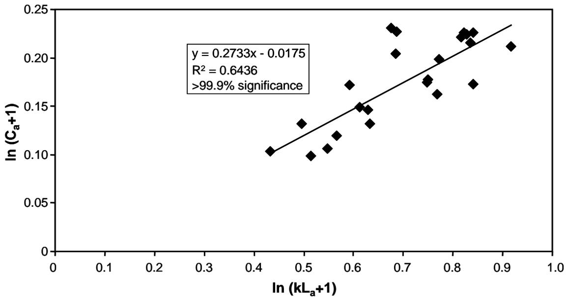
**Fig. 2.** Verification of equation 2 for **unbleached kraft** pulp high-consistency refined under atmospheric and pressurized conditions
