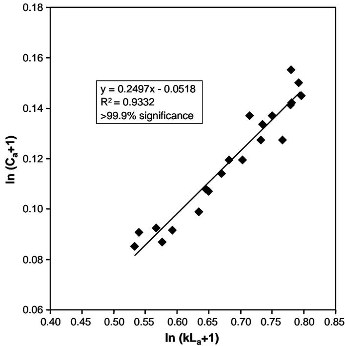
**Fig.1.** Verification of equation 2 for **unbleached kraft** pulp refined in an atmospheric high-consistency refiner
