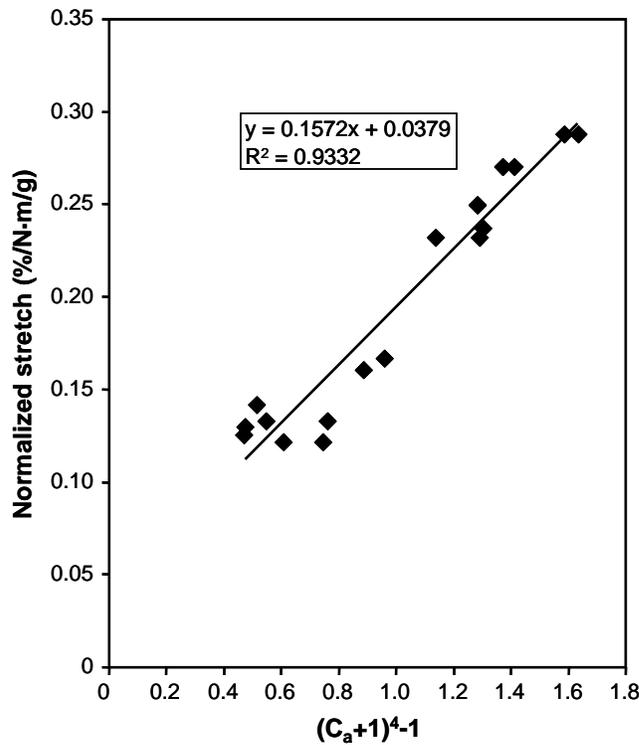
**Fig. 5.** Normalized stretch is plotted against  $(C_a + 1)^4 - 1$  for **bleached kraft** pulp refined under atmospheric and pressurized conditions.
