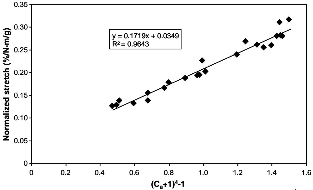
**Fig. 4.** Normalized stretch (stretch divided by tensile index) is plotted against  $(C_a + 1)^4 - 1$ , where  $C_a$  is the arithmetic curl index. This expression is assumed to be proportional to the number of microcompressions per fibre as explained in equation 3. The data are for **unbleached kraft** pulp refined under atmospheric and pressurized conditions.
