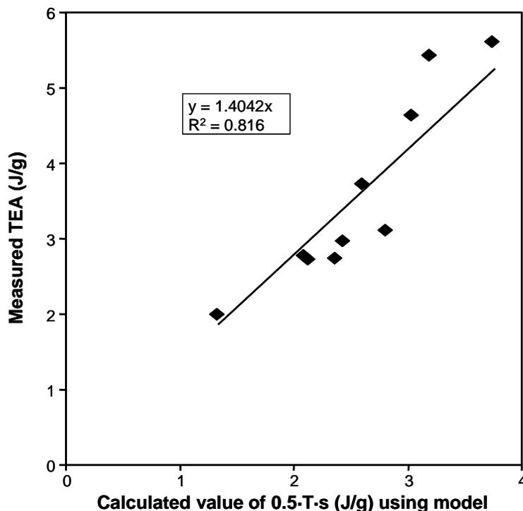
**Fig. 14.** To verify the ability of our model to predict the *TEA* of a pulp, the model was applied using equations 11 and 12 to the data set of another HCR trial based on a more recent sample of bleached kraft pulp.
