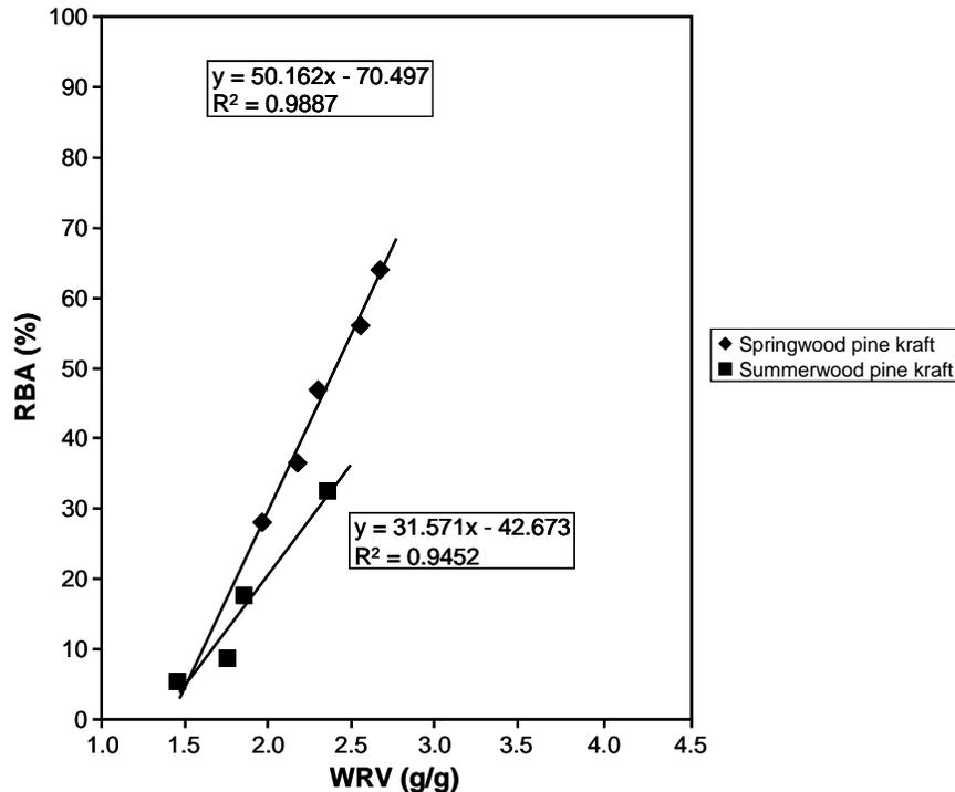
**Fig. 6.** Relative bonded area (*RBA*) is plotted against water retention value (*WRV*) for springwood and summerwood pine kraft pulps (Paavilainen 1990).
