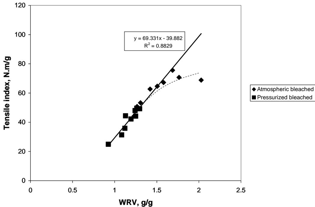
**Fig. 8.** A plot of tensile strength against *WRV* for **bleached kraft** pulp refined under atmospheric and pressurized conditions is also linear. The flattening off of the curve at high *WRV* is attributed to the limiting value of  $(8/9)Z$  according to the Page equation where *Z* is the zero-span tensile strength.
