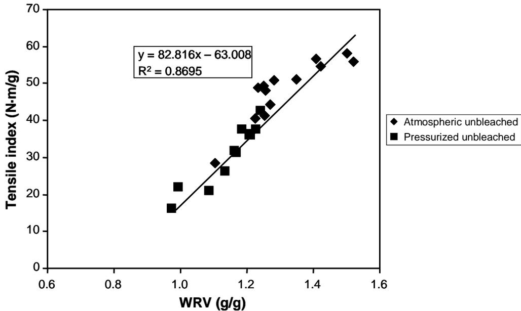
**Fig. 7.** Tensile strength is linearly correlated with *WRV* assuming that shear bond strength remains relatively constant with refining. The data are for **unbleached kraft** pulp refined under atmospheric and pressurized conditions.
