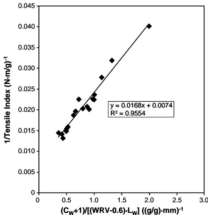
**Fig. 10.** A plot of equation 7 using data for **bleached kraft** pulp refined under atmospheric and pressurized conditions
