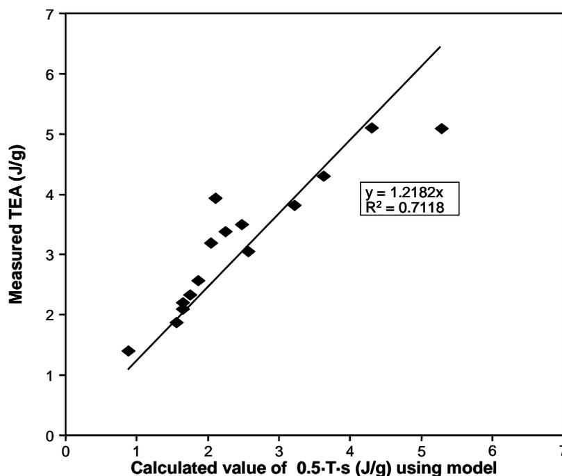
**Fig. 13.** The measured  $TEA$  index is plotted against a calculated  $TEA$  index using our model. The data are for **bleached kraft pulp** refined under atmospheric and pressurized conditions. The  $TEA$  index was calculated using equation 8 and the regression equations for  $s/T$  and  $1/T$  from Figs. 5 and 10 respectively (see equations 11 and 12).
