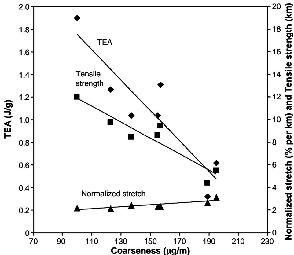
**Fig. 15.** The relationship between *TEA*, tensile, normalized stretch, and fibre coarseness is shown. Data were obtained from a study of pure wood species by Seth (1990).
