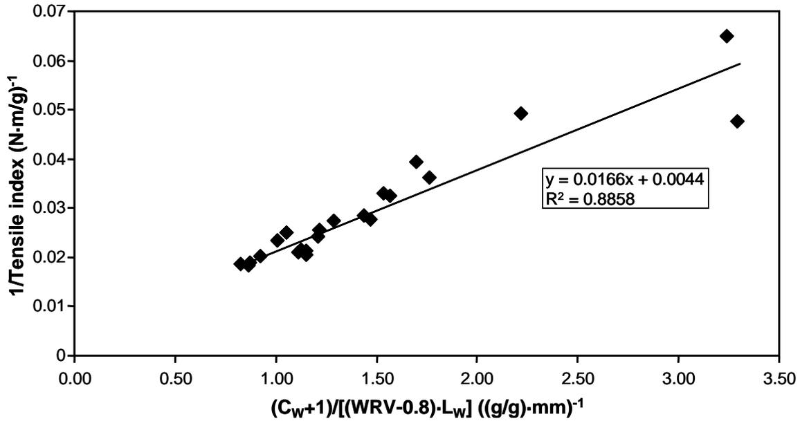
**Fig. 9.** A plot of equation 7 is shown relating tensile strength to length-weighted curl index  $C_w$ , length-weighted average fibre length,  $L_w$ , and  $WRV$  for **unbleached kraft** pulp refined under atmospheric and pressurized conditions.
