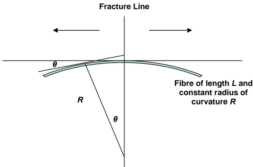
**Fig. A1.** Schematic drawing of curved fibre aligned in the direction of the applied stress
