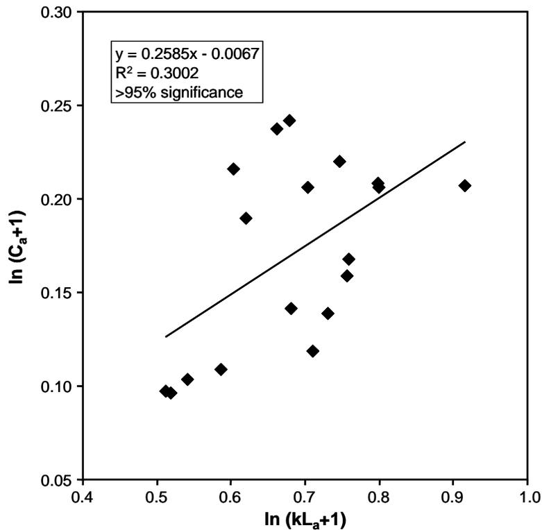
**Fig.3.** Verification of equation 2 for **bleached kraft** pulp high-consistency refined under atmospheric and pressurized conditions
