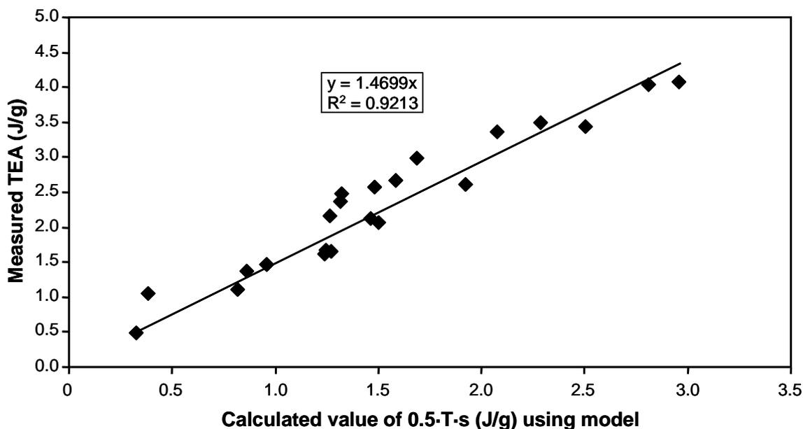
**Fig. 12.** This plot shows the measured  $TEA$  index against a calculated  $TEA$  index using our model. The  $TEA$  index was calculated using equation 8 and the regression equations for  $s/T$  and  $1/T$  from Figures 4 and 9 respectively (see equations 9 and 10). The data are for **unbleached kraft** pulp refined under atmospheric and pressurized conditions.
