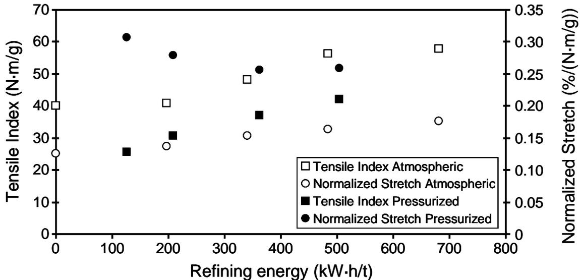
**Fig.16.** Effect of specific refining energy on normalized stretch and tensile index for atmospheric and pressurized HCR pulps.
