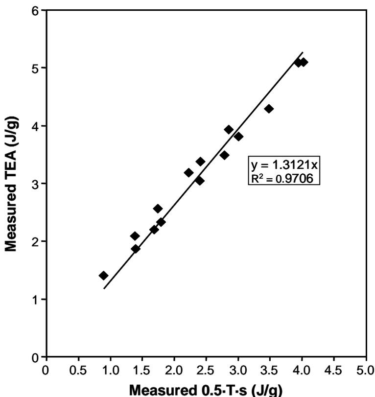
**Fig. 11.** The measured *TEA* index is plotted against the product of tensile index and stretch or elongation (elongation is expressed as a ratio, not as a percentage). The data are for **unbleached kraft** pulp refined under atmospheric and pressurized conditions.
