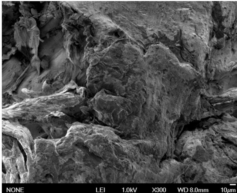
**Figure 11.** SEM micrograph of the 35% raw RH filler composite
