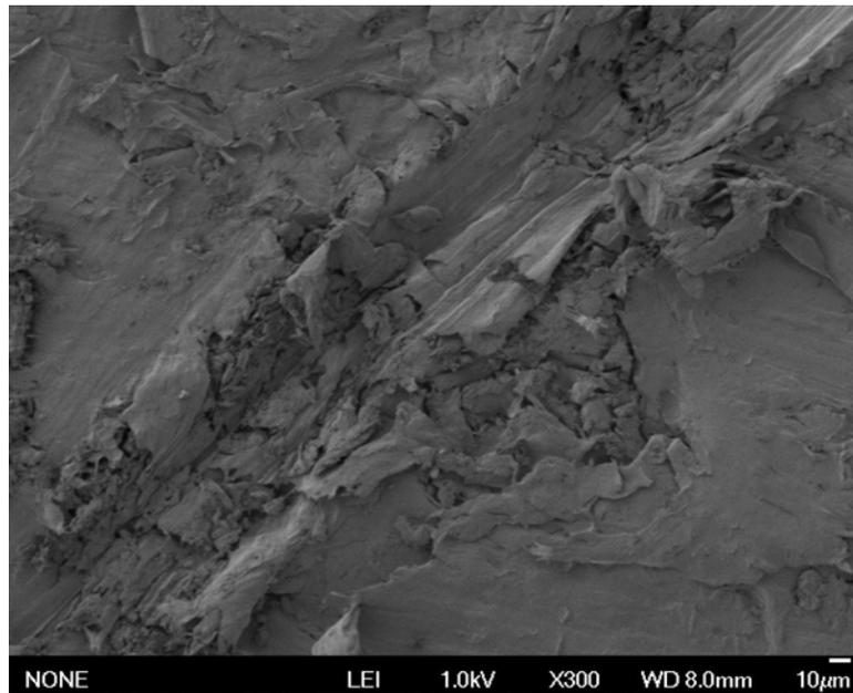
**Figure 12.** SEM micrograph of the 35% neutral media treated RH filler composite
