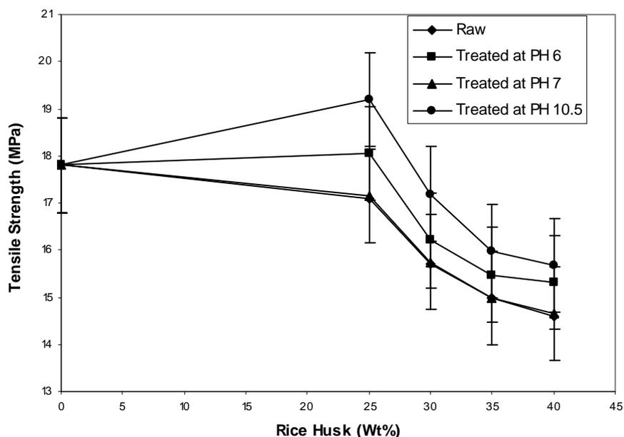
**Figure 1.** Variation of tensile strength at different filler loading
