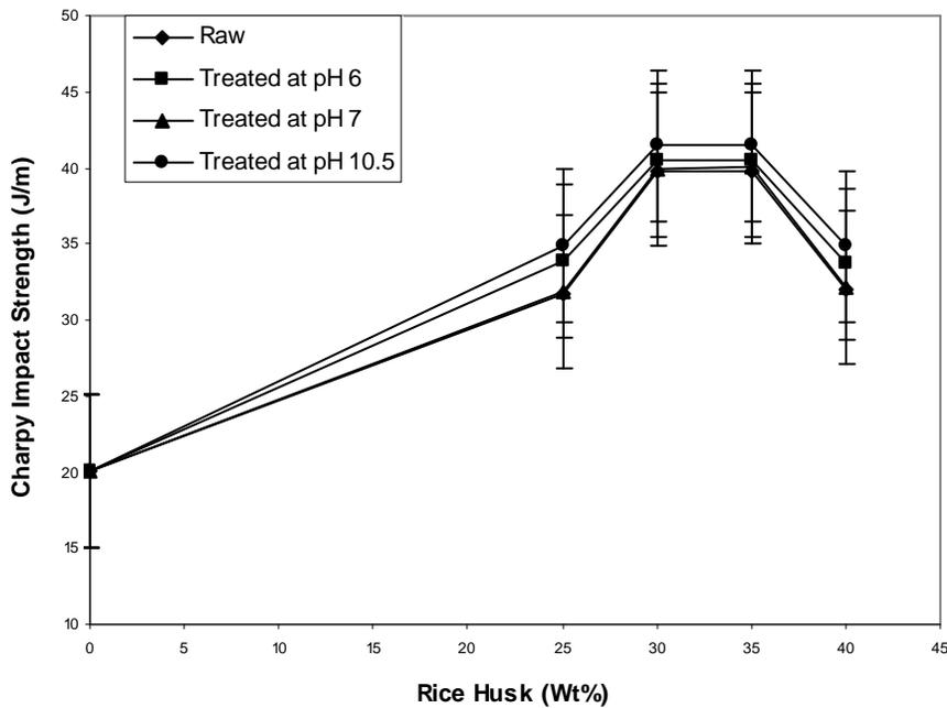
Figure 7. Variation of impact strength at different filler loading
