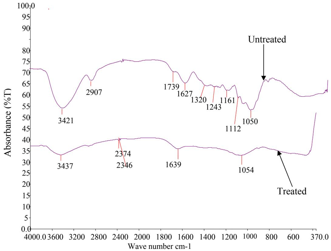
Figure 3. FT-IR spectra of untreated and treated rice husk
