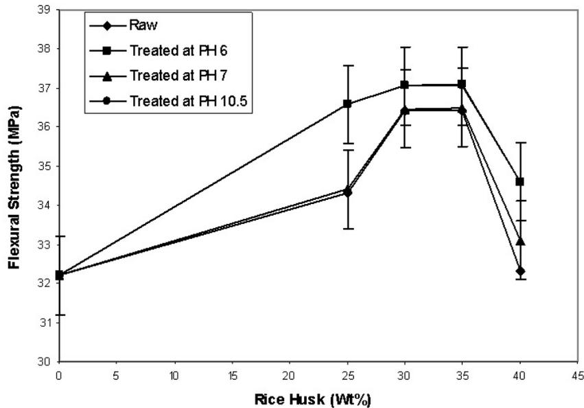
Figure 5. Variation of flexural strength at different filler loading
