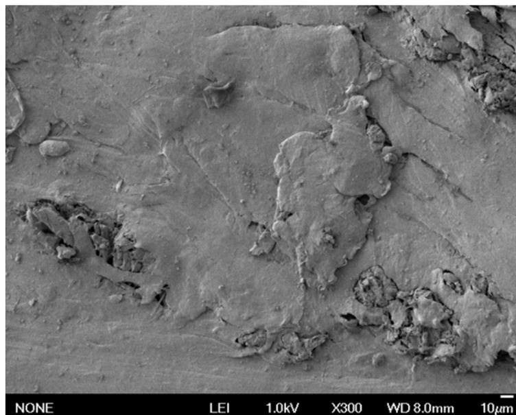
**Figure 13.** SEM micrograph of the 35% acidic media treated RH filler composite
