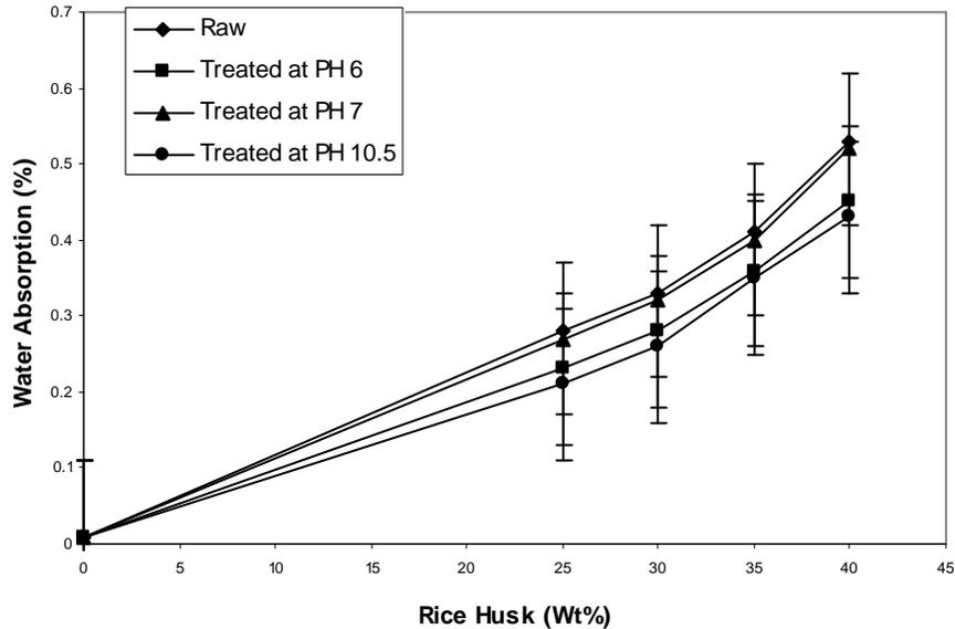
Figure 9. Variation of water absorption at different filler loadings immersed in cold water
