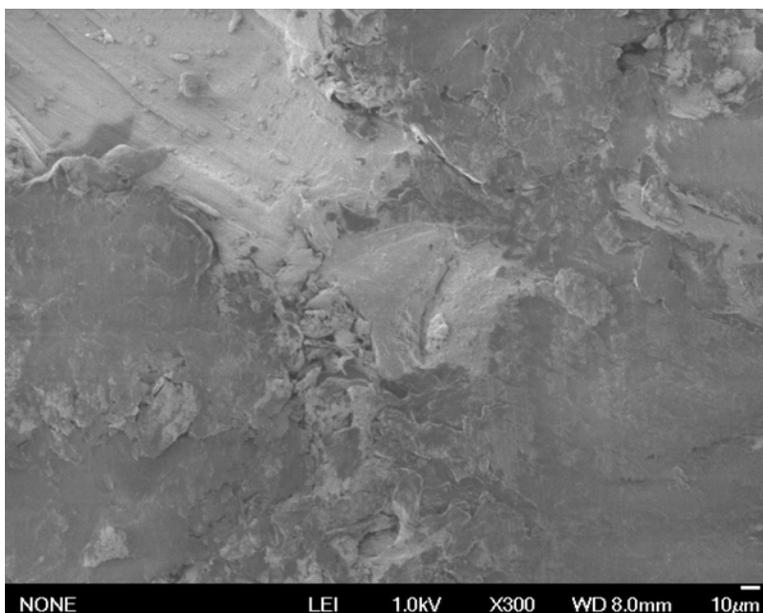
**Figure 14.** SEM micrograph of the 35% alkali media treated RH filler composite
