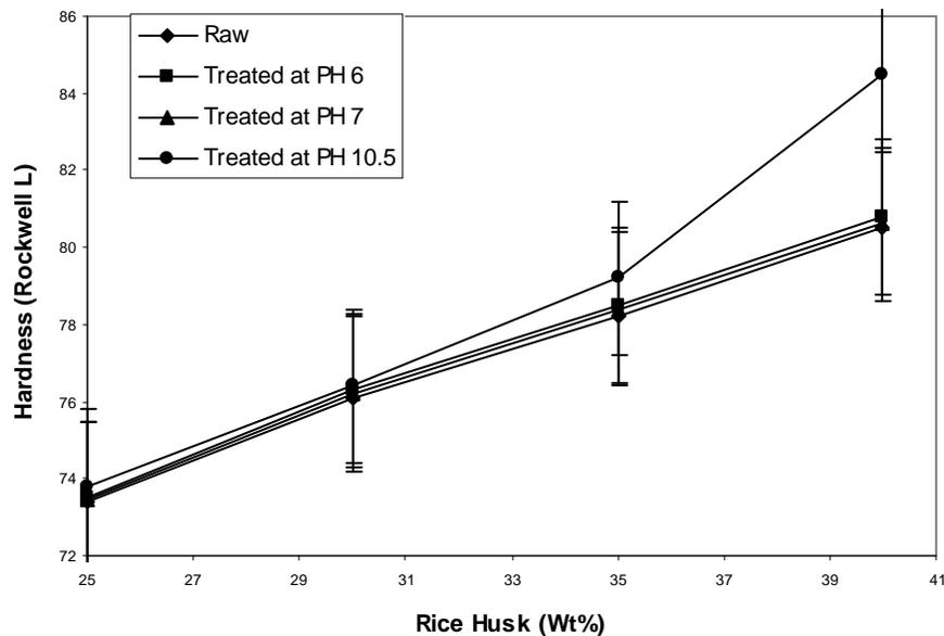
Figure 8. Variation of hardness at different filler loadings
