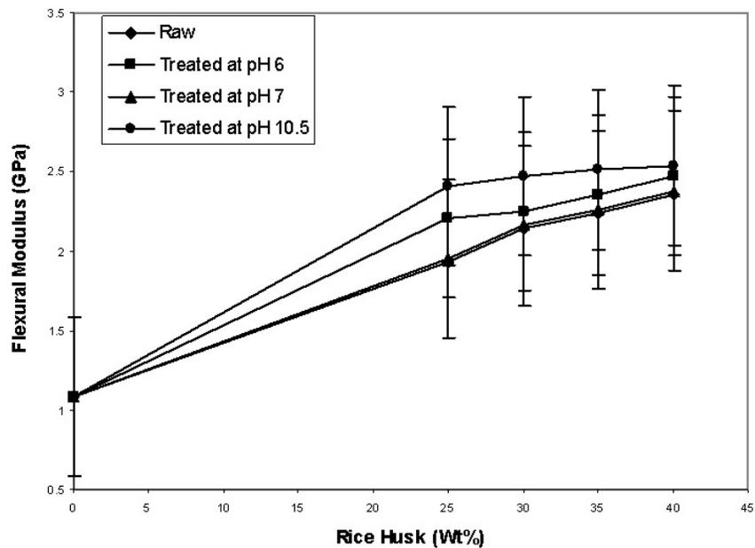
Figure 6. Variation of flexural modulus at different filler loading
