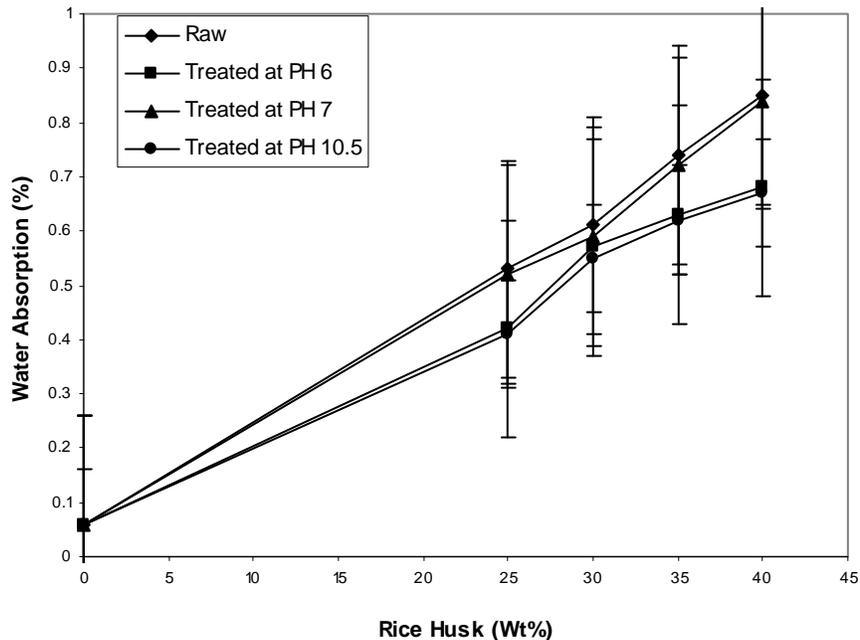
Figure 10. Variation of water absorption at different filler loadings immersed in hot water
