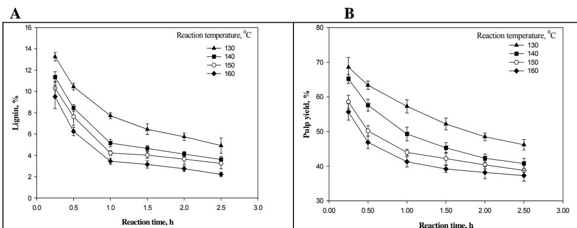
**Fig. 1.** Curves of different reaction times vs (A) lignin, and (B) pulp yield at different cooking temperature during soda pulping of sugarcane bagasse
