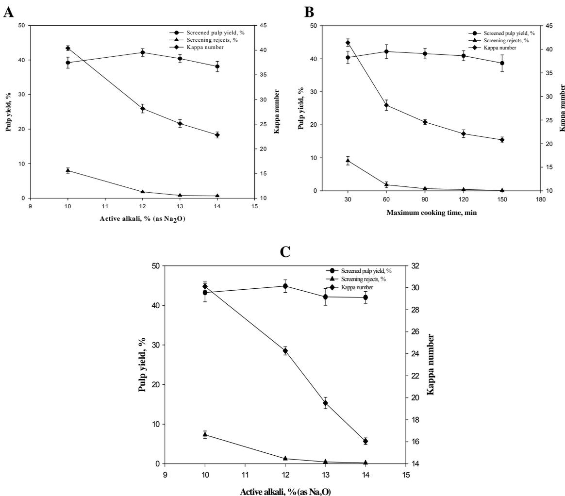
**Fig. 2.** Effect of (A) active alkali, (B) maximum cooking time, and (C) AQ dose at different alkali doses on screened pulp yield, screening rejects, and kappa number during soda pulping of sugarcane bagasse
