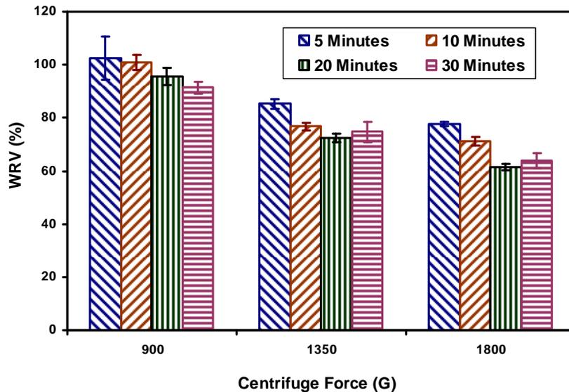
**Fig. 4.** Water retention values of MCC (0.5 g) with varied centrifugal times and varied relative centrifugal forces
