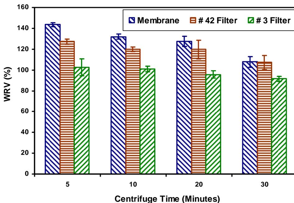
**Fig. 5.** Water retention values of MCC (0.5 g) with different filter paper/membranes at varied centrifugal times (relative centrifugal forces: 900 G).
