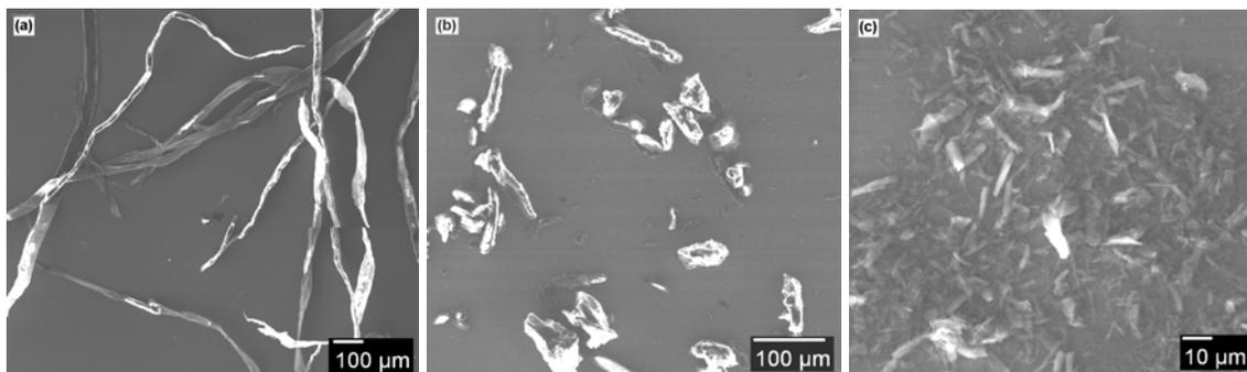
**Fig. 1.** SEM images of pulp fibers (a), MCC (b), and treated MCC using a homogenizer with 138 MPa pressure and 20 passes (c)
