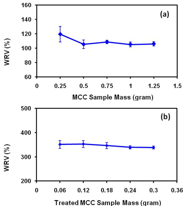
**Fig. 3.** WRVs with standard deviations of MCC with centrifugal force of 900 G and time of 5 min (a) and treated MCC with centrifugal force of 900 G and time of 20 min (b) at varied specimen masses
