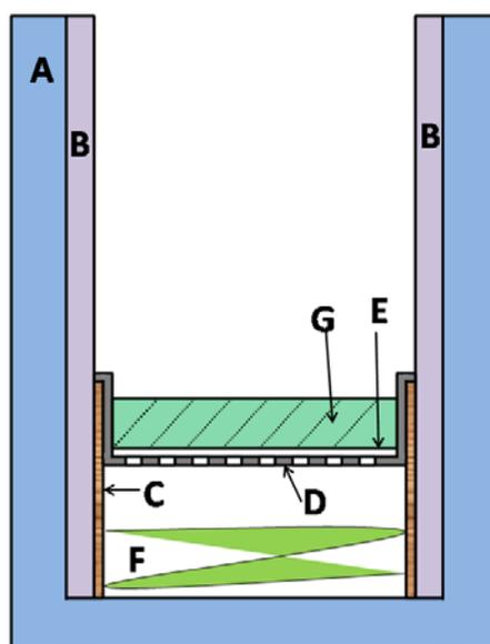
**Fig. 2.** Scheme of water retention value measurement setup for centrifuge, A: Centrifuge bucket, B: Adapter, C: Spacer, D: Stainless steel cap with holes, E: Filter paper/Membrane, F: Tissue for water absorption, G: Sample
