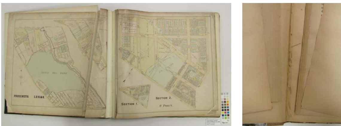
Figure 2. Examples of acidic printed items that have failed at the fold. Left: Atlas with acidic paper. Right: Brittle pages separating from a binding
