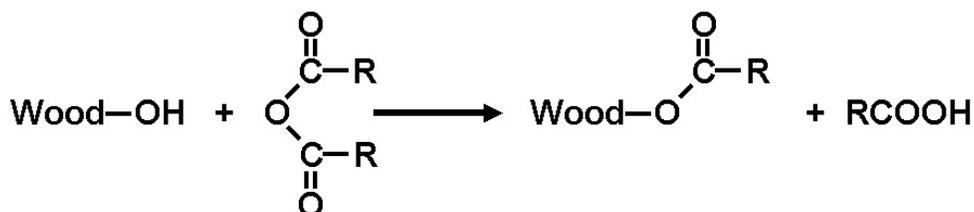
**Fig. 1.** Anhydride modification scheme, where R = CH<sub>3</sub> (acetic anhydride), and R = C<sub>2</sub>H<sub>5</sub> (propionic anhydride)
