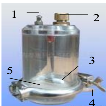
Fig. 1. Apparatus for evaluation of ultrafiltration characteristics: 1 - Connection of the steel bottle to a source of N_2 to maintain the pressure; 2 - Feeding hole; 3 - Rotor; 4 - Discharging hole; 5 - Ultrafiltration membrane
