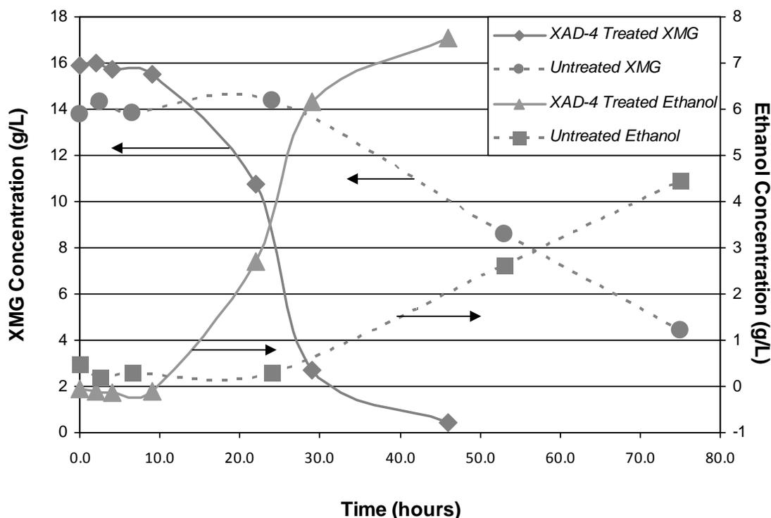
**Fig. 3.** Consumption of xylose/mannose/galactose and ethanol production in both XAD-4 treated (solid lines) and untreated (dashed lines) samples. Arrows indicate which plot accompanies which axis.
