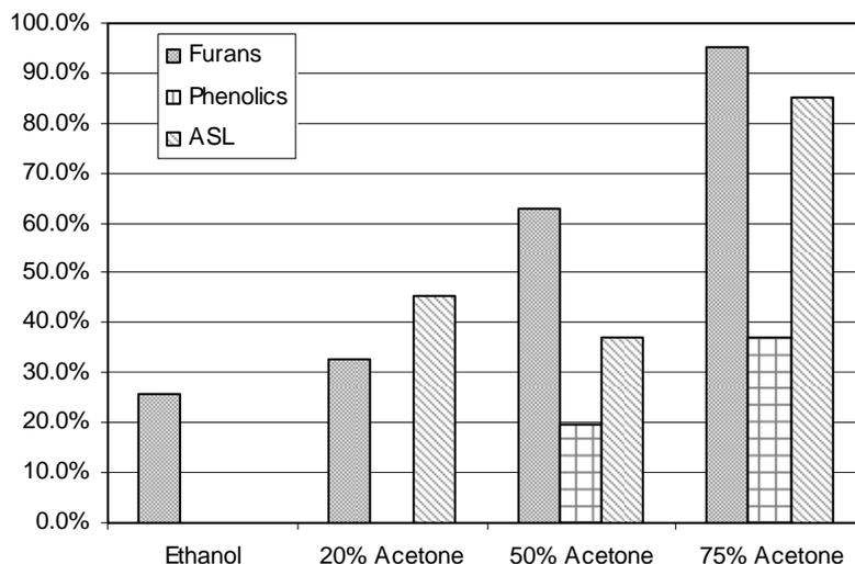
**Fig. 2.** Recovery of furans, phenolic monomers, and acid-soluble lignin (ASL) using various solvents. Note that the ability of ethanol to remove ASL was not investigated.
