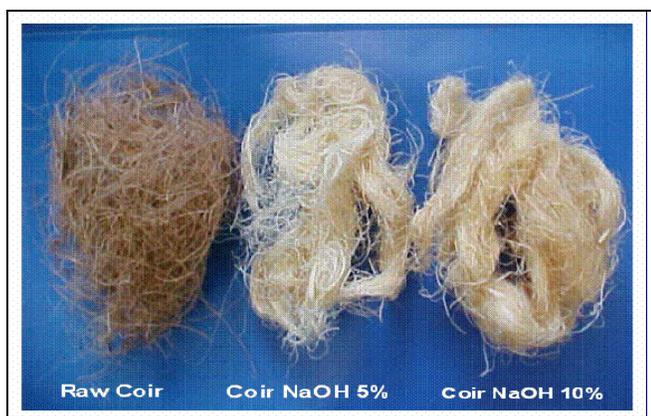
**Fig. 2.** Dwarf-green coir fibers before and after alkali treatment
