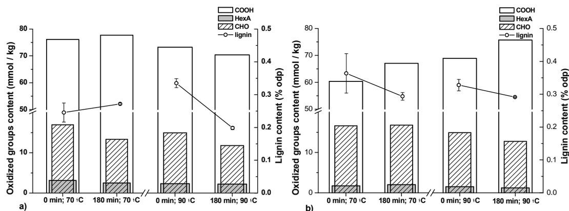
**Fig. 4.** Content of oxidized groups and of residual lignin during hydrogen peroxide final bleaching of **a)**  $D_0(EOP)D_1$  and **b)**  $OQ(PO)D$  partially bleached pulps. Final P stage conditions: 2.0% odp  $H_2O_2$ ; 0.6-0.9% odp NaOH; 0.05% DTPA; 70-90°C; 0-180 min.
