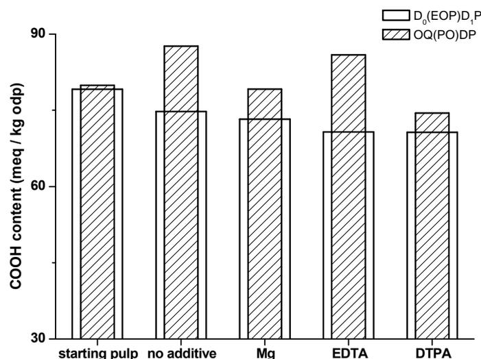
**Fig. 3.** Effect of hydrogen peroxide stabilizers added in a final P stage on the content of carboxyl groups of D<sub>0</sub>(EOP)D<sub>1</sub>P and OQ(PO)DP fully bleached pulps
