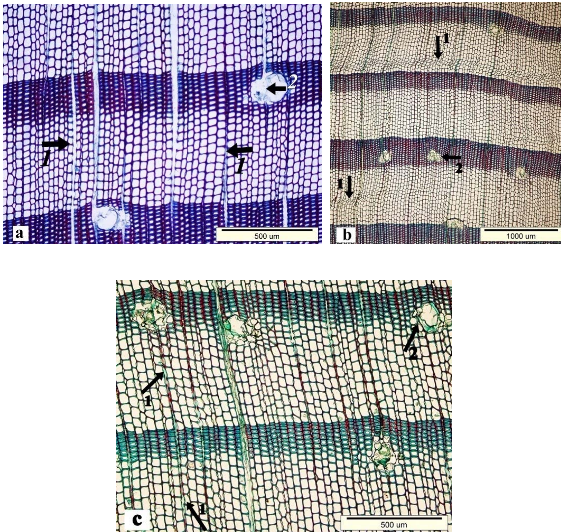
Fig. 3. a) No visible distortion in the plane of growth rings, radial cracks along the rays (arrows 1), axial resin canals in circular shape and damaged epithelial cells around these canals (arrows 2) in Group A, b) Buckling on the radial cell walls of the earlywood tracheids and wavy pattern in relevant regions (arrow 1), and axial canals in circular shape (arrow 2) in Group B, c) Slight shift in radial direction of the growth rings, rays in narrow nodular shape (arrow 1), axial resin canals almost in circular shape and damaged epithelial cells around these canals (arrow 2) in Group C
