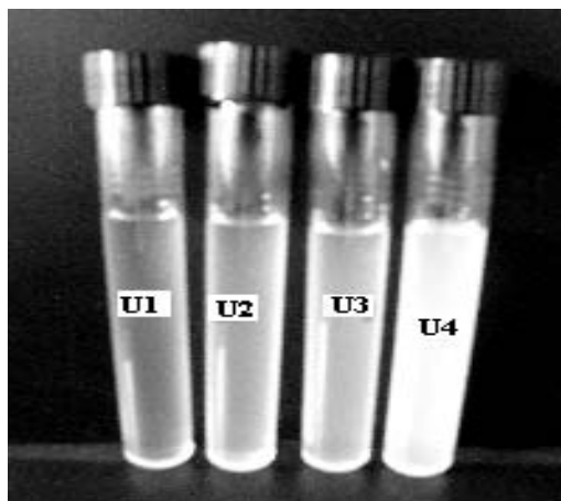
Fig. 1. Cellulose nanofibers (U1...U4 samples) obtained by ultrasonication treatment
