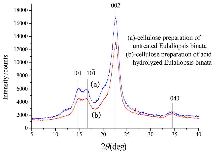
Fig.4. X-ray diffraction of cellulose preparations
