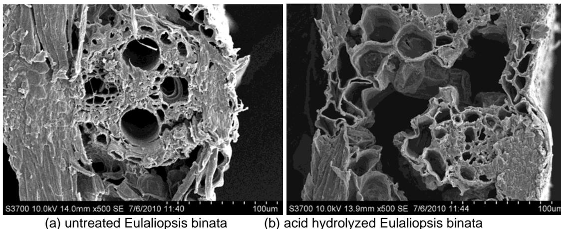
**Fig. 1.** SEM photographs of the cross section
