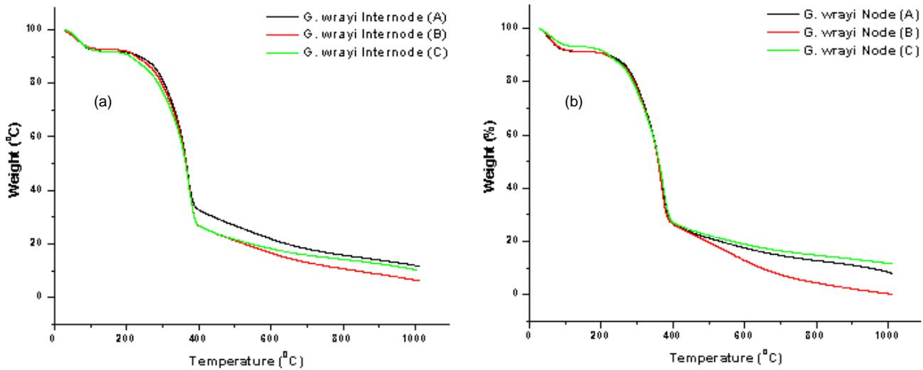
**Figure 4.** Thermogravimetric analysis of *Gigantochloa wrayi* internode (a), and node (b)
