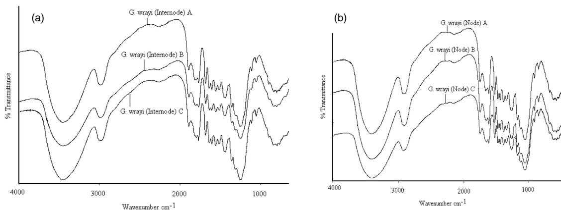
**Figure 2.** FTIR spectra of *Gigantochloa wrayi* internode (a), and node (b)
