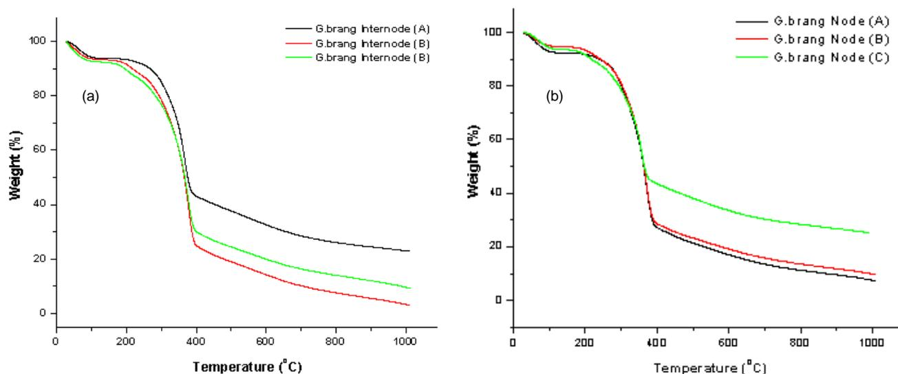
**Figure 3.** Thermogravimetric analysis of *Gigantochloa brang* internode (a), and node (b)
