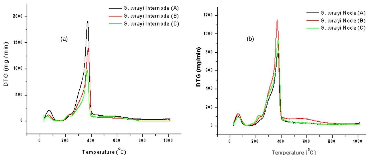
**Figure 6.** DTG analysis of *Gigantochloa wrayi* internode (a), and node (b)
