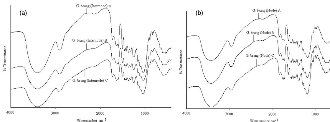
**Figure 1.** FTIR spectra of *Gigantochloa brang* internode (a), and node (b)
