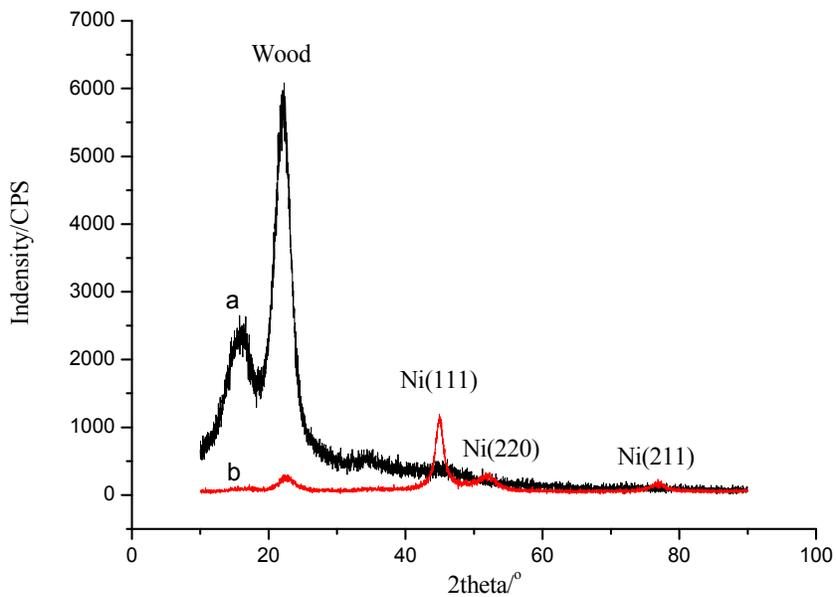
**Figure 5.** XRD patterns of the pristine (a) and the plated wood veneer (b)
