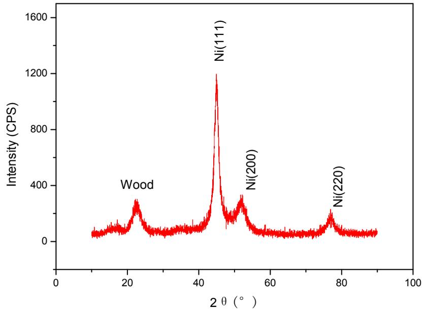
**Figure 4.** XRD pattern of the plated wood veneer
