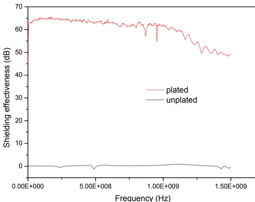
**Figure 6.** Electromagnetic shielding effectiveness of wood veneers before and after plating
