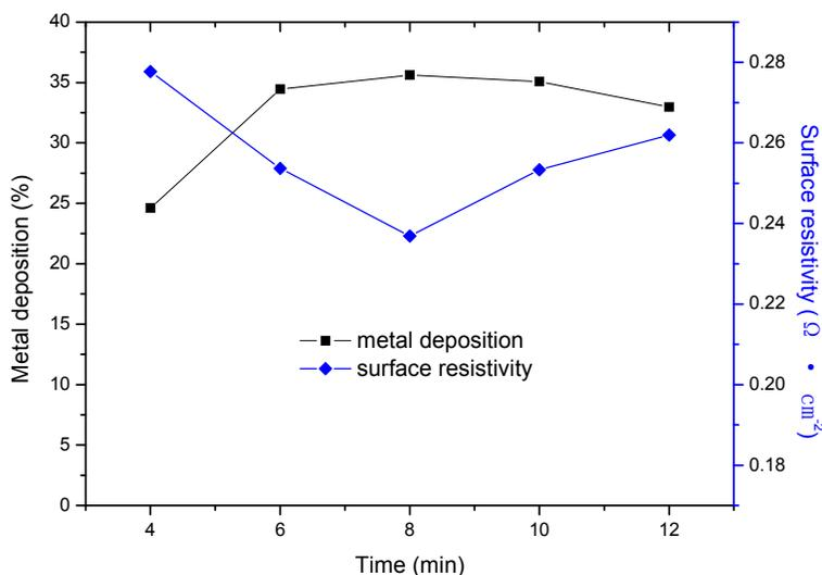
**Figure 1.** Influence on metal deposition and surface resistivity by the coordination between chitosan and Pd (II)
