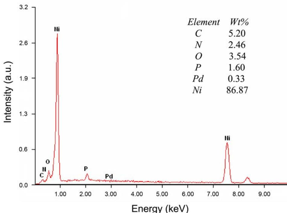
**Figure 3.** EDS spectra of the plated wood veneer
