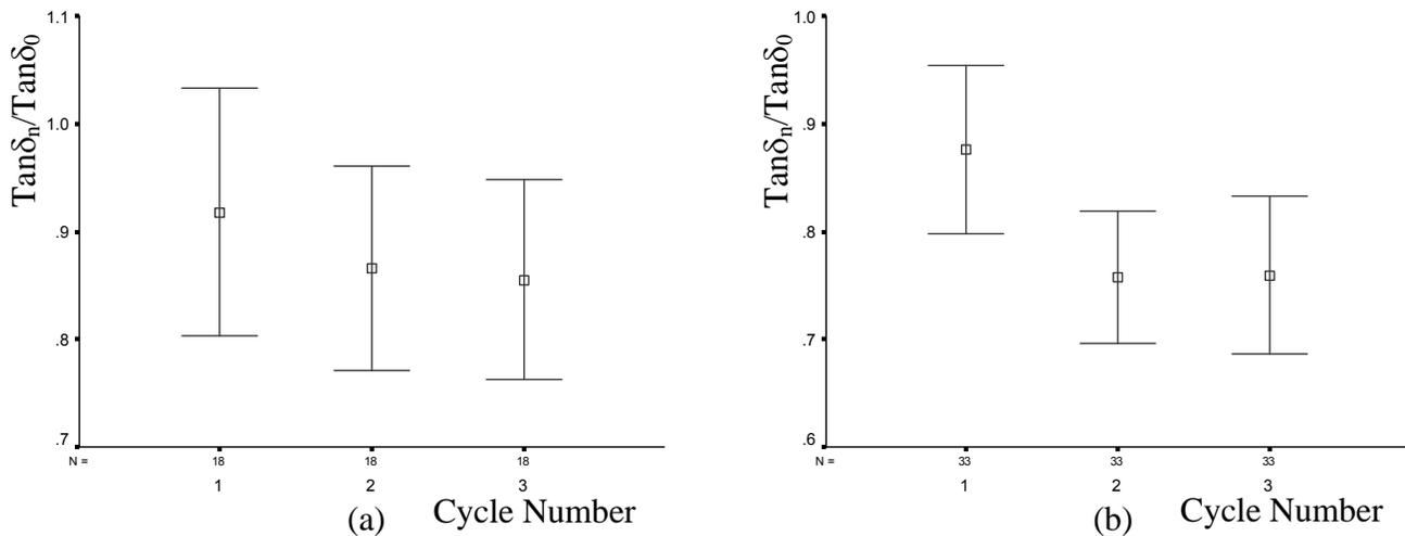
**Fig. 2.** Effect of soaking cycles on the mean value of the damping coefficient ratio ( $\tan\delta_n / \tan\delta_0$ ) for (a) Mulberry and (b) Walnut. With  $\tan\delta_n$ : damping coefficient after  $n^{\text{th}}$  soaking cycle and  $\tan\delta_0$ : damping coefficient of the preliminary unsoaked specimens. Standard deviations marked by the error bars
