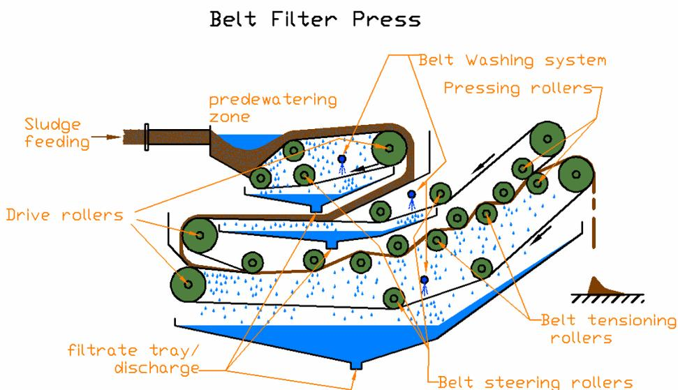
**Fig. 1.** Schematic illustration of the belt filter press
