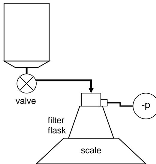
**Fig. 2.** Schematic illustration of the laboratory drainage device
