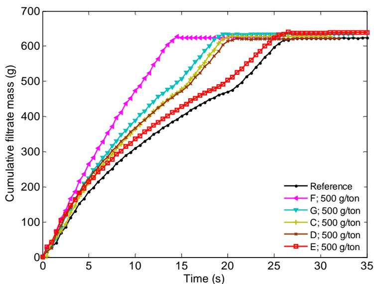
Fig. 6. Cumulative filtrate mass as a function of time for polymer dosage of 0.5 kg/ton
