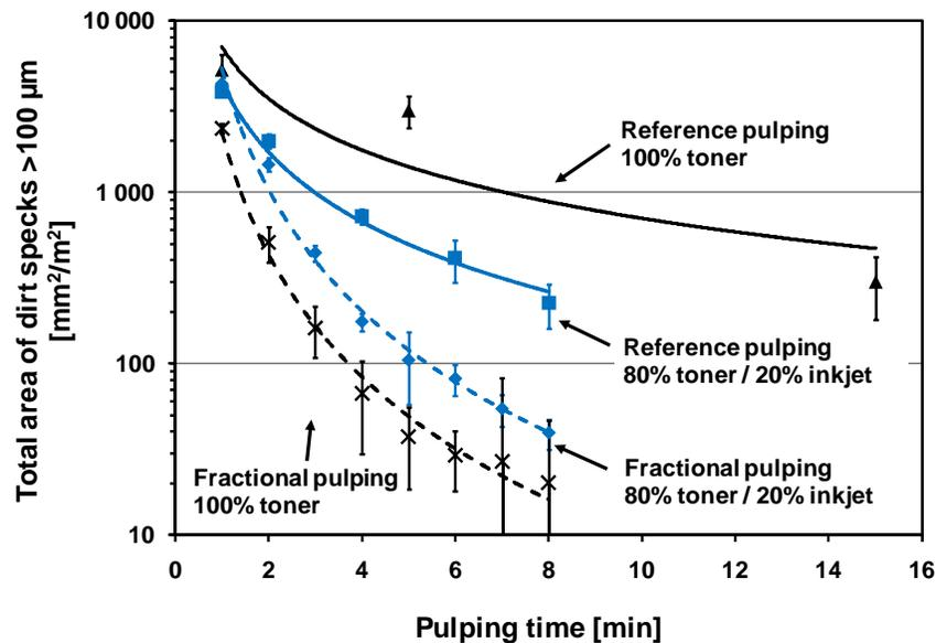
**Fig. 6.** The total area of large dirt specks (>100  $\mu\text{m}$ ) as a function of pulping time when pulping 100% toner printed papers, and an 80/20 mixture of toner/inkjet papers conventionally and with a fractional pulping approach. The error bars represent the confidence interval for a 95% confidence level.
