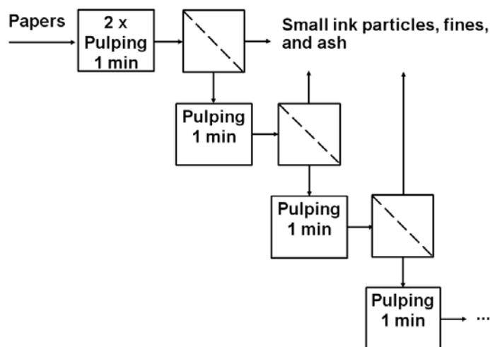
**Fig. 2.** A schematic drawing of the fractional pulping procedure
