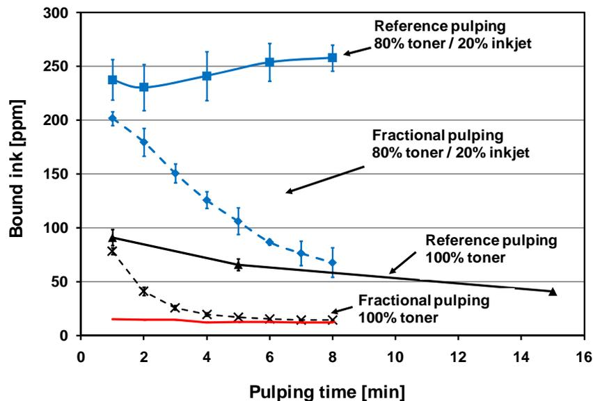
**Fig. 4.** Ink bound to fibers as a function of pulping time when pulping 100% toner printed papers, and an 80/20 mixture of toner/inkjet printed papers in a conventionally and with the fractional pulping approach. The red solid line on the bottom represents the hyperwashed residual ink content of unprinted paper which is free of ink. The error bars represent the confidence interval for a 95% confidence level.
