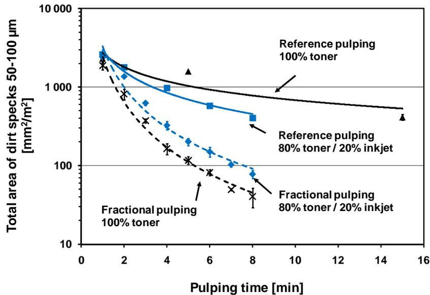
**Fig. 5.** The total area of small dirt specks (50-100  $\mu\text{m}$ ) as a function of pulping time when pulping 100% toner printed papers, and an 80/20 mixture of toner/inkjet papers conventionally and with a fractional pulping approach. The error bars represent the confidence interval for a 95% confidence level.
