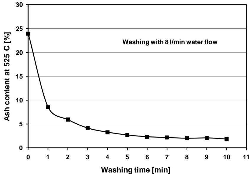
**Fig. 1.** Ash content of pulp made of unprinted paper as a function of washing time (water flow 8 l/min) in a Sommerville device equipped with 150-mesh wire screen. Residual ash (approximately 2%) is considered to be bound to fibers and thus not removable by the washing treatment.
