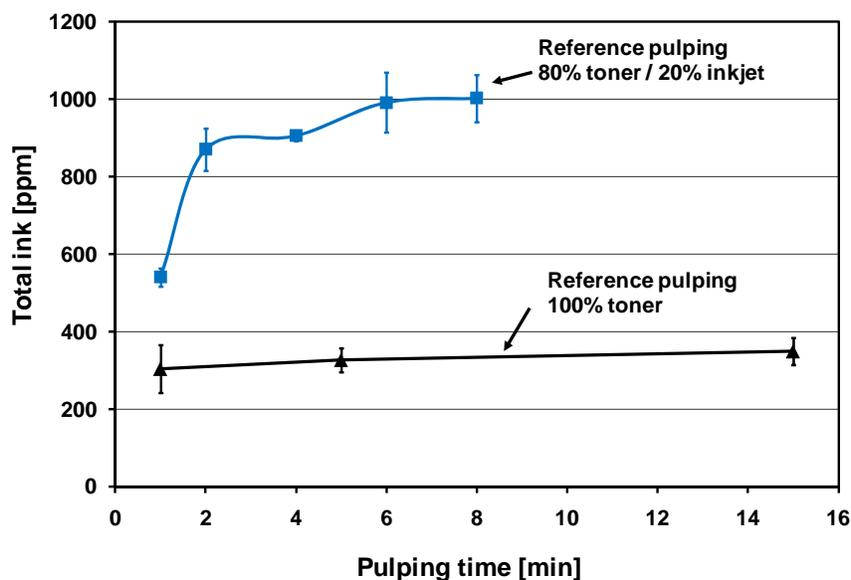
**Fig. 3.** Total ink content as a function of pulping time in conventional pulping when pulping 100% toner printed papers and an 80/20 mixture of toner/inkjet printed papers. The error bars represent the confidence interval for a 95% confidence level.
