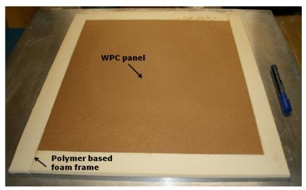
Fig. 1. A sample of the WPC panel containing the FR
