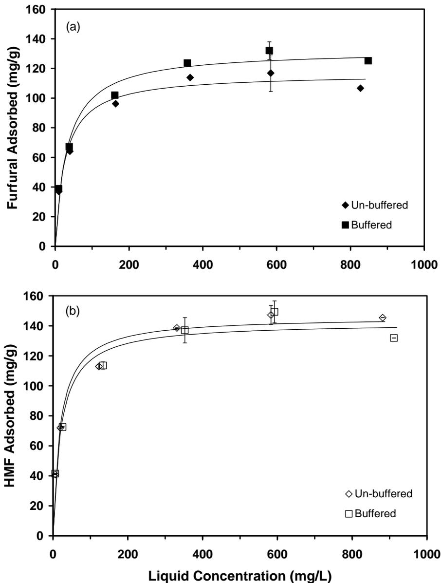
**Fig. 2.** Results of isotherm study using either furfural or HMF in buffered or un-buffered sugar solutions in contact with steam-activated flax shive chars. Curves represent best fit using the Langmuir isotherm correlation.
