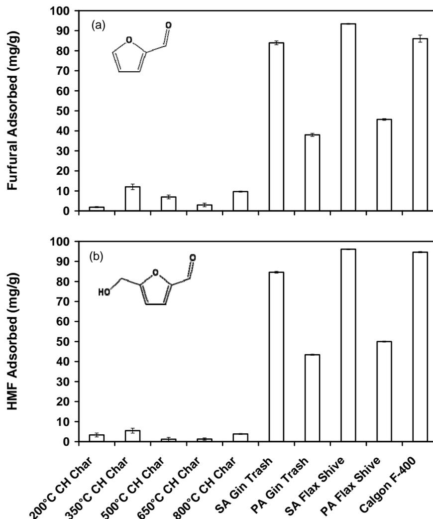
**Fig. 1.** Adsorption of furfural (a) and HMF (b) from water by cotton seed hull (CH) chars and steam (SA) or phosphoric acid (PA) activated gin trash or flax shive chars. A commercial product (Calgon F-400) is included for comparison. Error bars correspond to standard deviation values from results of triplicate experiments.
