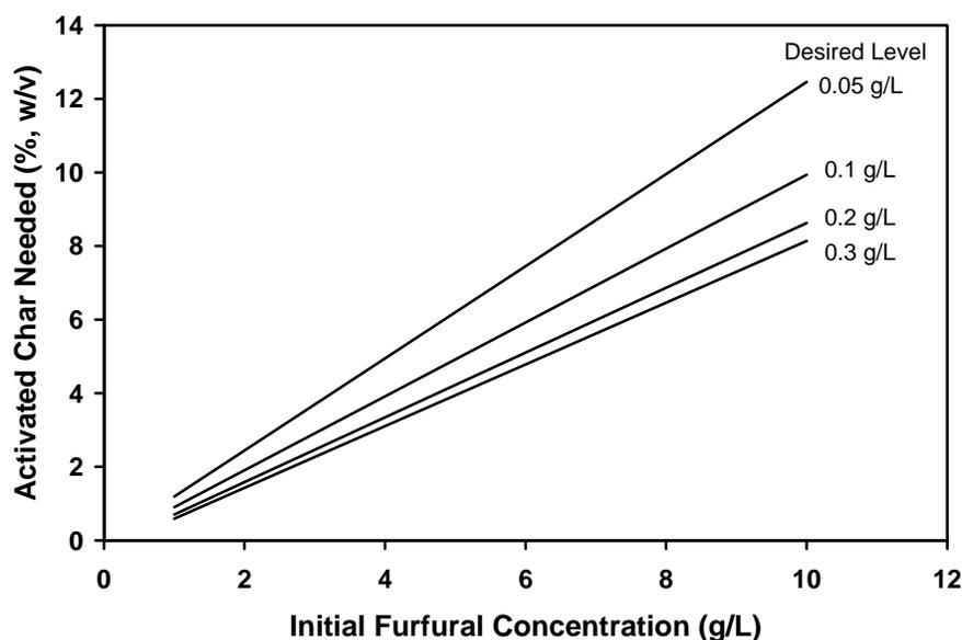
**Fig. 3.** Estimated steam activated char dosing requirement to remove furfural to a desired level ( $q_m=132$ ,  $k=0.0305$ ).
