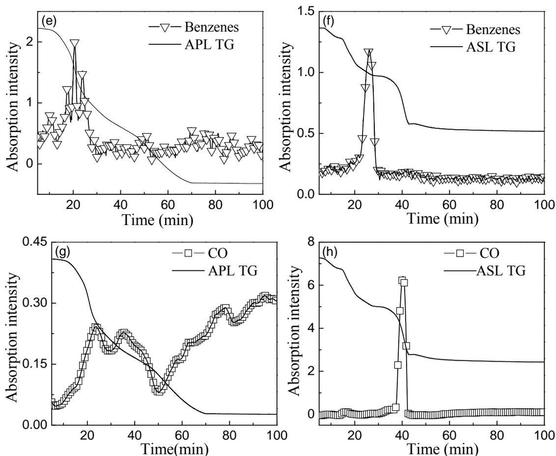
Fig. 8B. FTIR profiles of gas product evolving from APL and ASL pyrolysis and gasification
