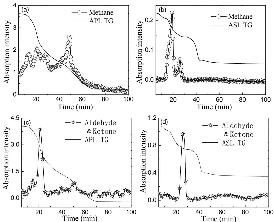
**Fig. 8A.** FTIR profiles of gas product evolving from APL and ASL pyrolysis and gasification
