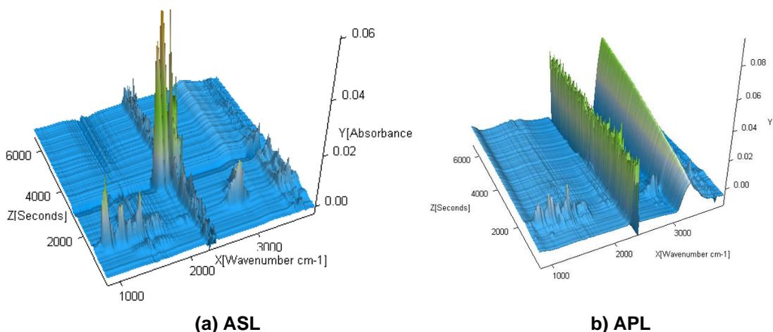
**Fig. 5.** 3D FTIR spectra from pyrolysis and CO<sub>2</sub> gasification of ASL and APL
