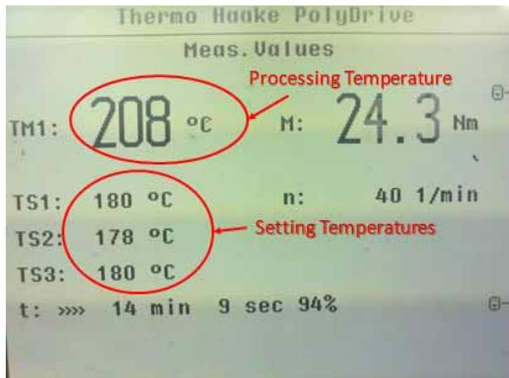
**Fig. 6.** Difference between setting temperatures and processing temperature
