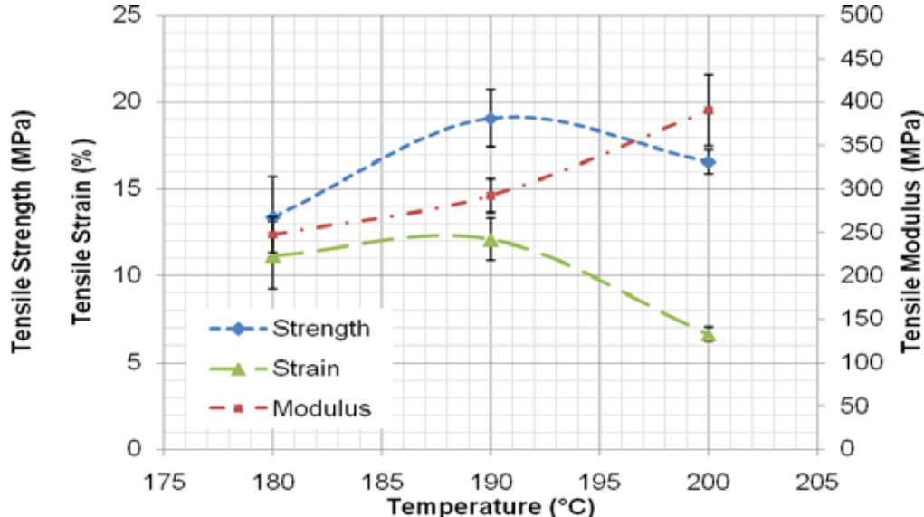
**Fig. 5.** Effect of processing temperature on tensile properties of TPU/KF composite
