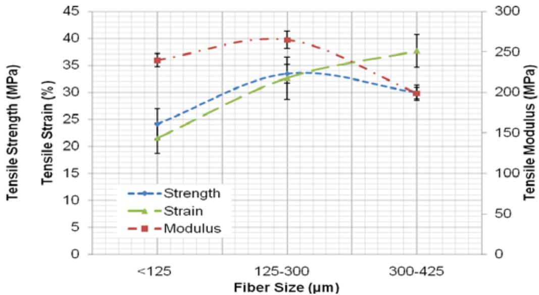
**Fig. 9.** Effect of fiber size on tensile strength of TPU/KF composite
