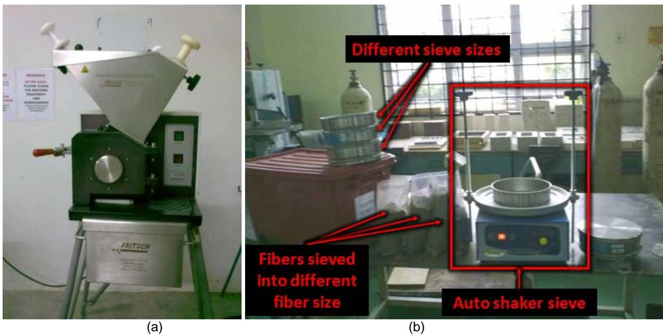
**Fig. 2.** (a) Mill used to pulverize the fibers, (b) Auto shaker sieve
