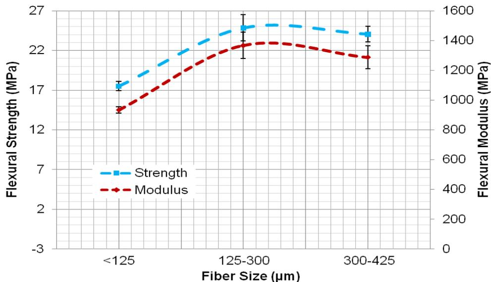
**Fig. 10.** Effect of fiber size on flexural properties of TPU/KF composite
