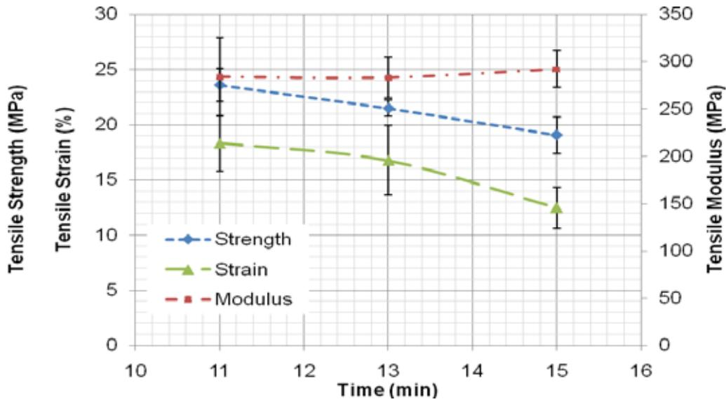
Fig. 7. Effect of processing time on tensile properties of TPU/KF composite
