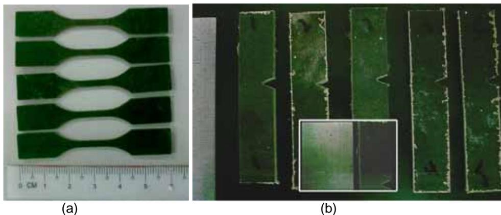
**Fig. 4.** (a) Tensile specimens , (b) Impact specimens
