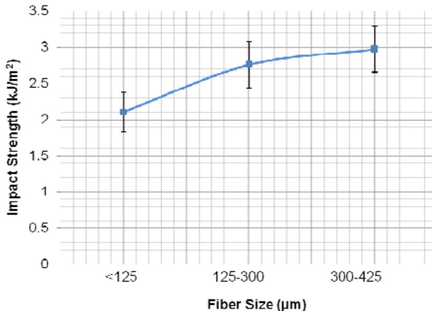
**Fig. 11.** Effect of fiber size on impact strength of TPU/KF composite
