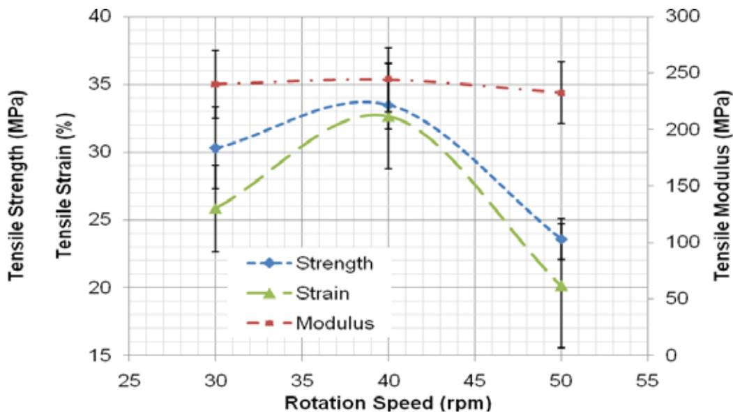
Fig. 8. Effect of processing speed on tensile strength of TPU/KF composite
