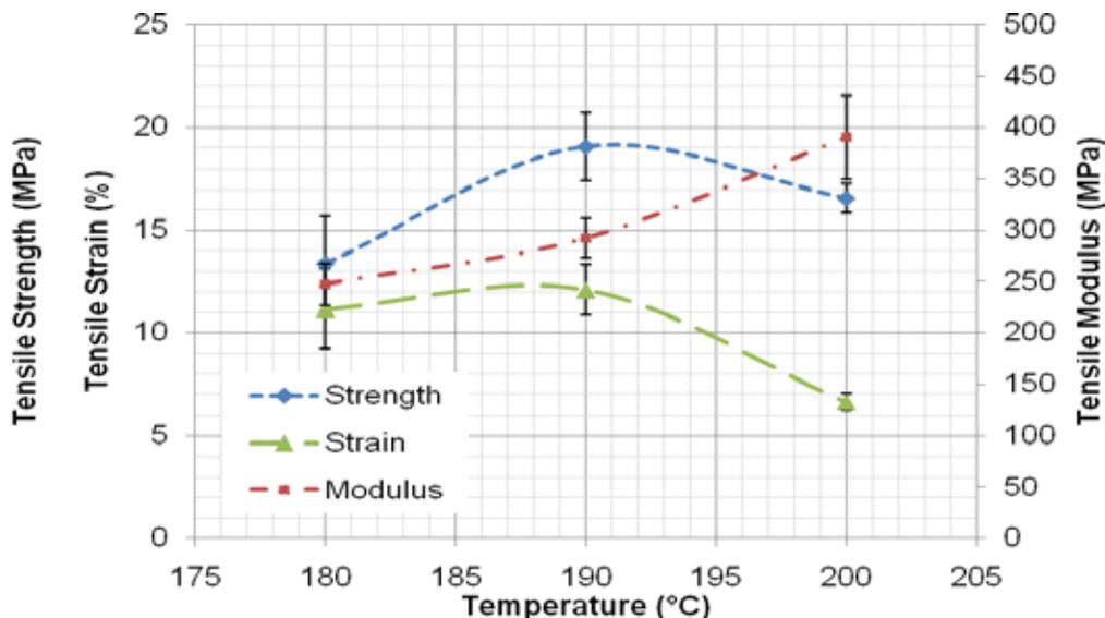
**Fig. 6.** Effect of processing temperature on tensile properties of TPU/KF composite
