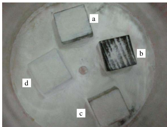
Fig.1. Comparison among different volumes of mycelium on Chinese white poplar specimens a: 5h, 215°C; b: 5h, 230°C; c: 5h, 200°C; d: 5h, 170°C
