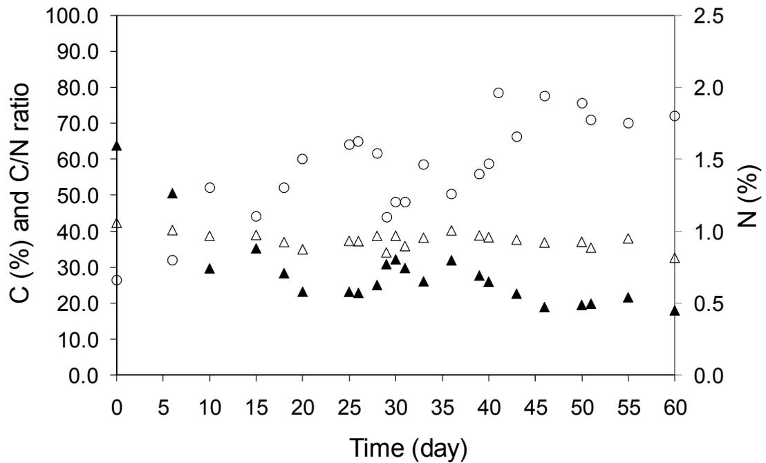
Fig. 4. Changes of carbon, nitrogen and C/N ratio throughout co-composting of CGOPF and POME anaerobic sludge. Remarks :  $\Delta$ = Carbon, O= Nitrogen and  $\blacktriangle$  = C/N ratio
