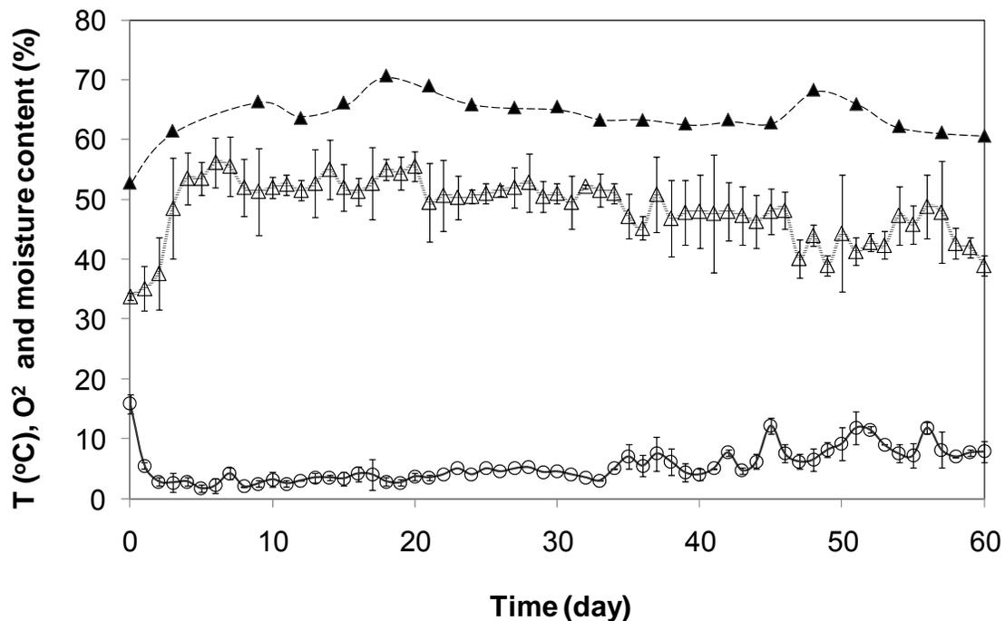
**Fig. 2.** Profiles of compost temperature, oxygen level and moisture content during co-composting of OPF and POME anaerobic sludge. Remarks:  $\Delta$  = Temperature, O = Oxygen content and  $\blacktriangle$  = Moisture content.
