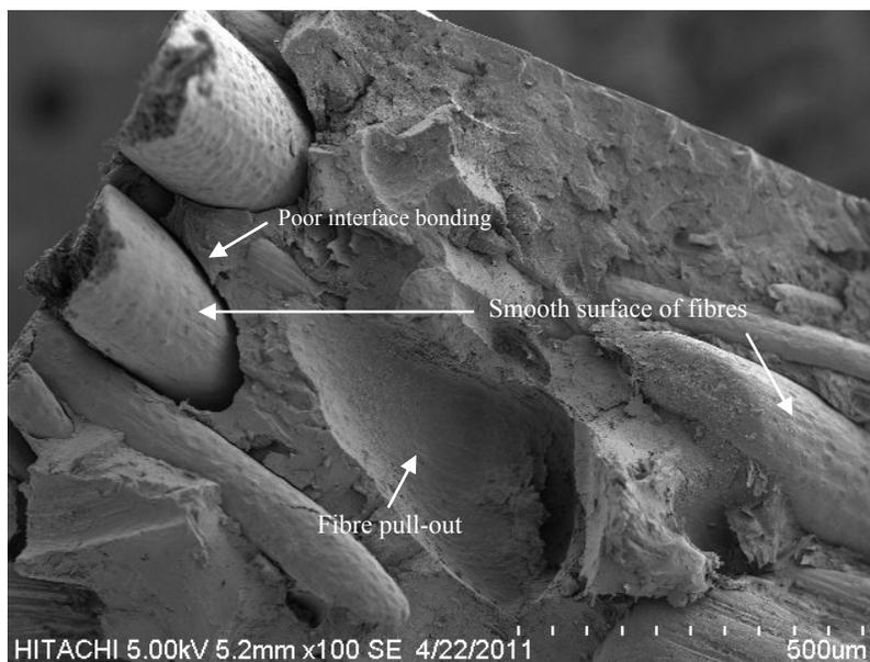
**Fig. 4.** The fracture surface of an untreated 40%SPF-HIPS composite
