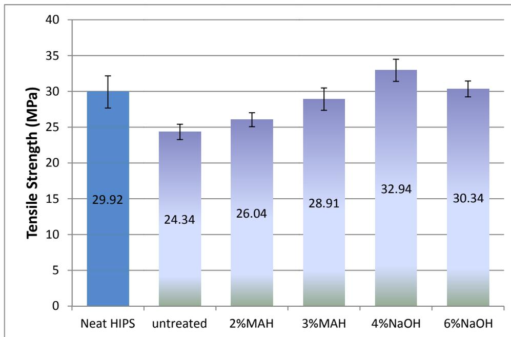
Fig. 2. Tensile strengths of untreated and treated of SPF-HIPS composites
