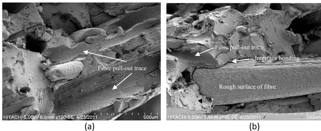
**Fig. 6.** The fracture surface of a SPF-HIPS composite treated with (a) 4% alkali, (b) 6% alkali
