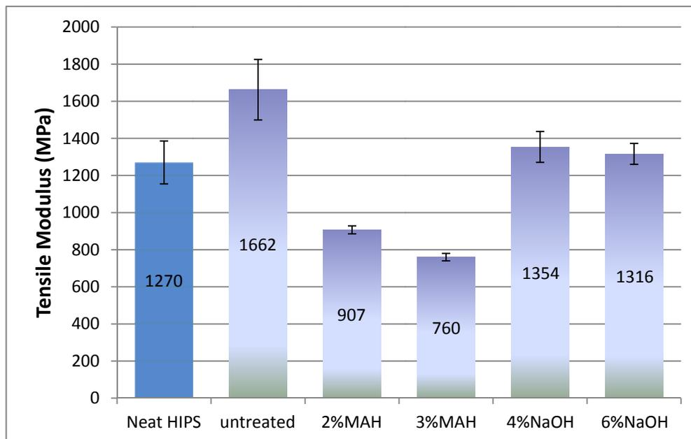
Fig. 3. Tensile moduli of untreated and treated SPF-HIPS composites
